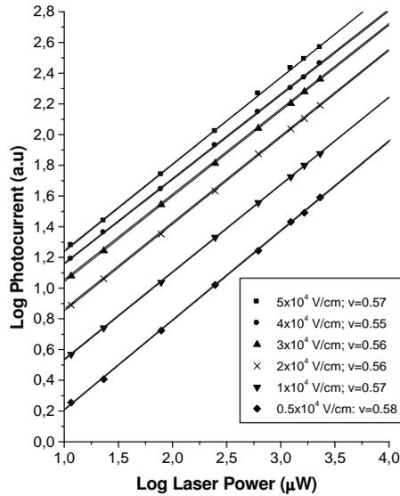
**Figure 4.** Excitation light intensity-dependence of photocurrent at various levels of applied electric fields. Data were taken at room temperature (290 K).
