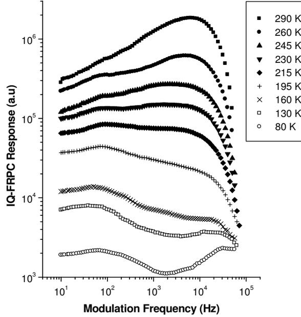
**Figure 1.** In-quadrature frequency-resolved photocurrent (IQ-FRPC) response of a-As<sub>2</sub>Se<sub>3</sub> at various temperatures. Excitation light intensity is 2.31 mW with the wavelength of 632.8 nm.
