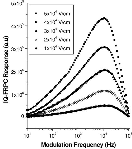
**Figure 2.** IQ-FRPC response of a-As<sub>2</sub>Se<sub>3</sub> under various applied electric fields. Excitation light intensity is 2.31 mW with the wavelength of 632.8 nm. Data were taken at room temperature (290 K).
