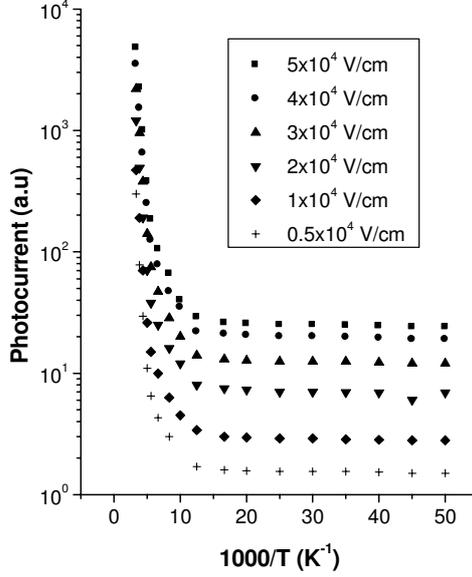
**Figure 3.** Photocurrent vs. inverse temperature at various levels of applied electric fields. Excitation light intensity is 2.31 mW with the wavelength of 632.8 nm.
