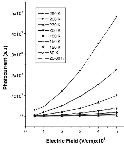
**Figure 5.** Electric field-dependence of photocurrent at various temperatures. Excitation light intensity was kept constant at 2.31 mW with the wavelength of 632.8 nm.
