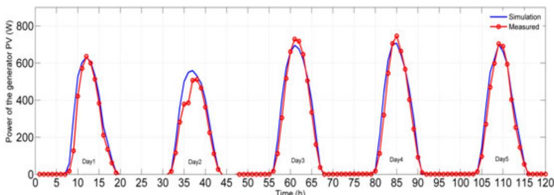
**Figure 7.** Comparison of measured output power (red) and simulation results (blue).
