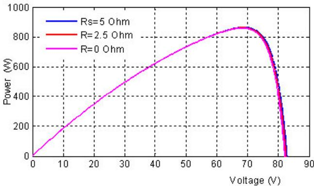
**Figure 5.** *P-V* characteristics of a module for different values of the series resistance  $R_s$ .
