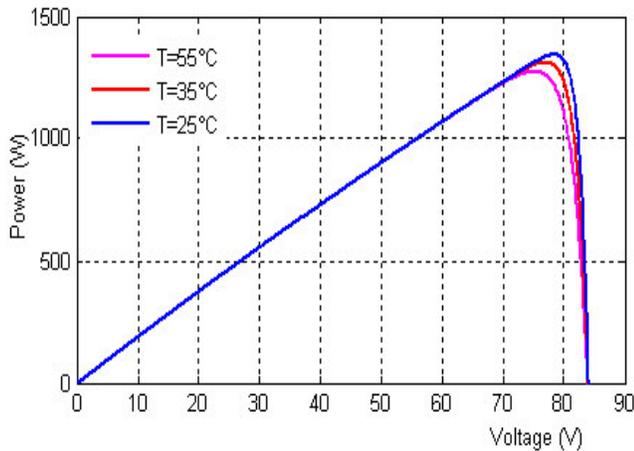
**Figure 3.** *P-V* characteristics of a module at different temperatures.
