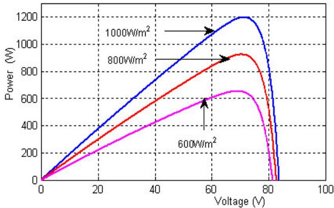
**Figure 2.** *P-V* characteristics for a module at 40°C, for several sunlight intensities.
