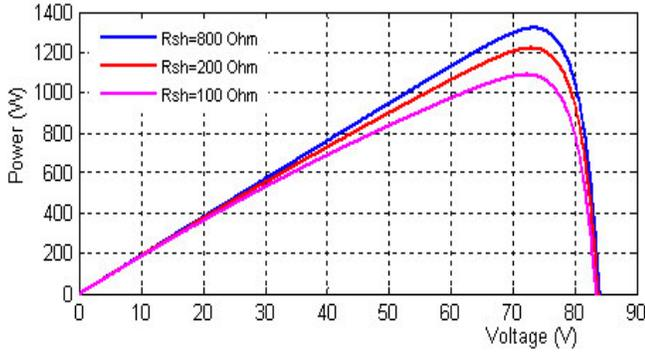
**Figure 4.** *P-V* characteristics of a module for different values of the shunt resistance  $R_{Sh}$ .
