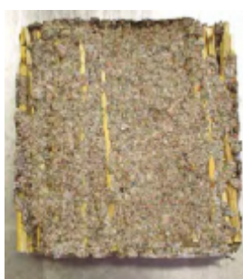
Figure 2a. Reed plates with a cellulose flake binder
