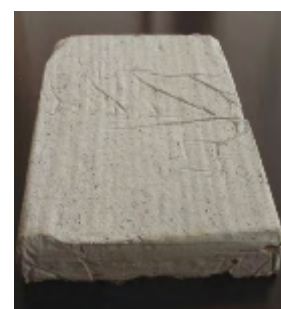
Figure 2d. Reed plates with a lime mortar binder
