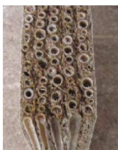
Figure 2b. Reed plates with a natural resin glue binder
