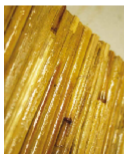
Figure 2c. Reed plates with a maize binder
