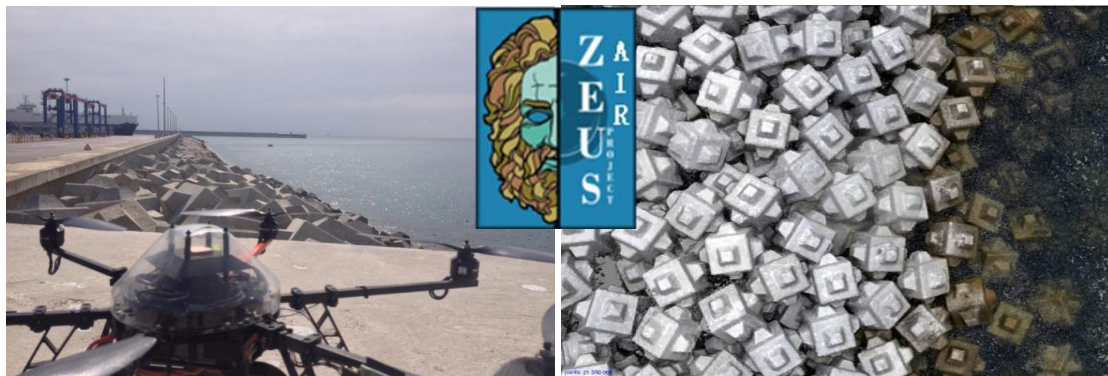
Figure 1. Dron equipped with zeus-air (left) and scanned detail (right) of the new breakwater of San Andrés (Málaga) made with Cubipods. Images given by the company Flyviews.
