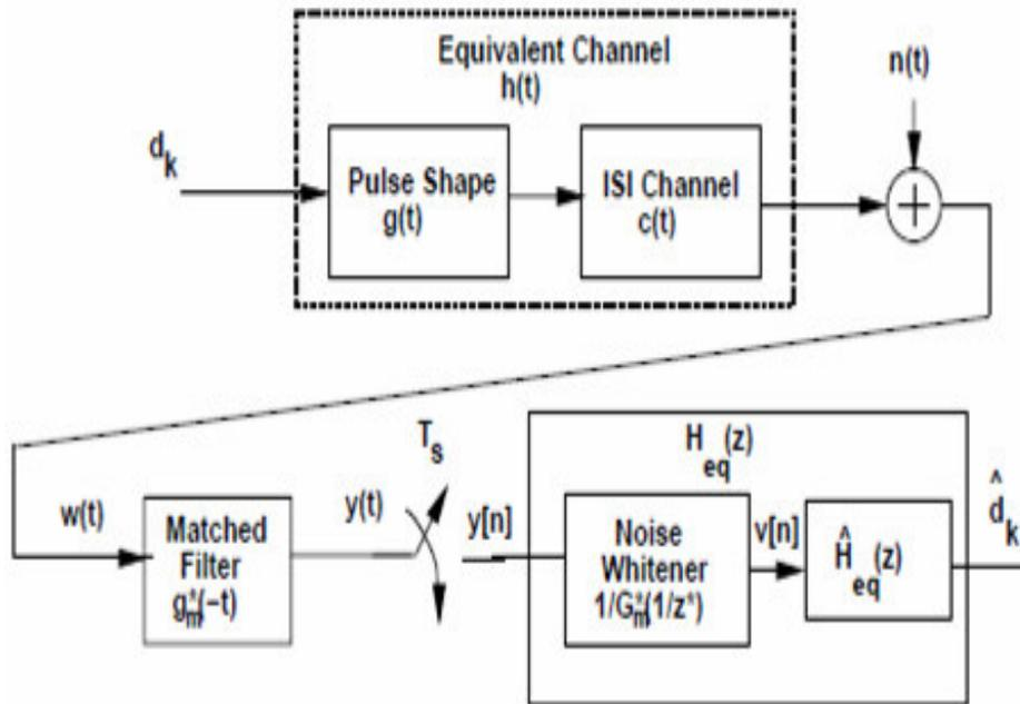
Figure 3. MMSE equalizer with noise whitening filter.
