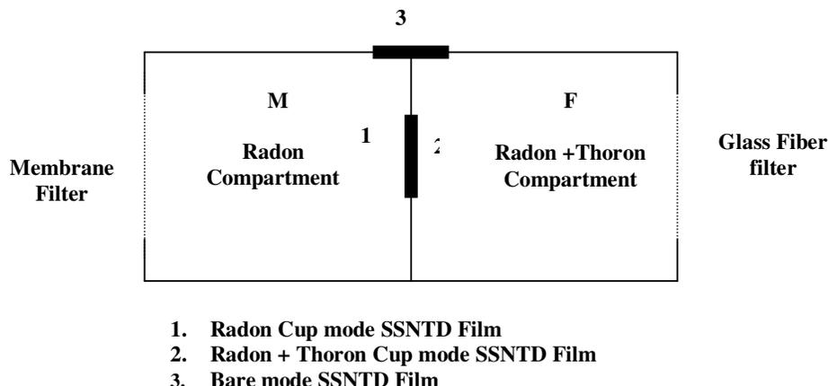
**Figure 2.** Schematic of twin cup radon-thoron dosimeter.
