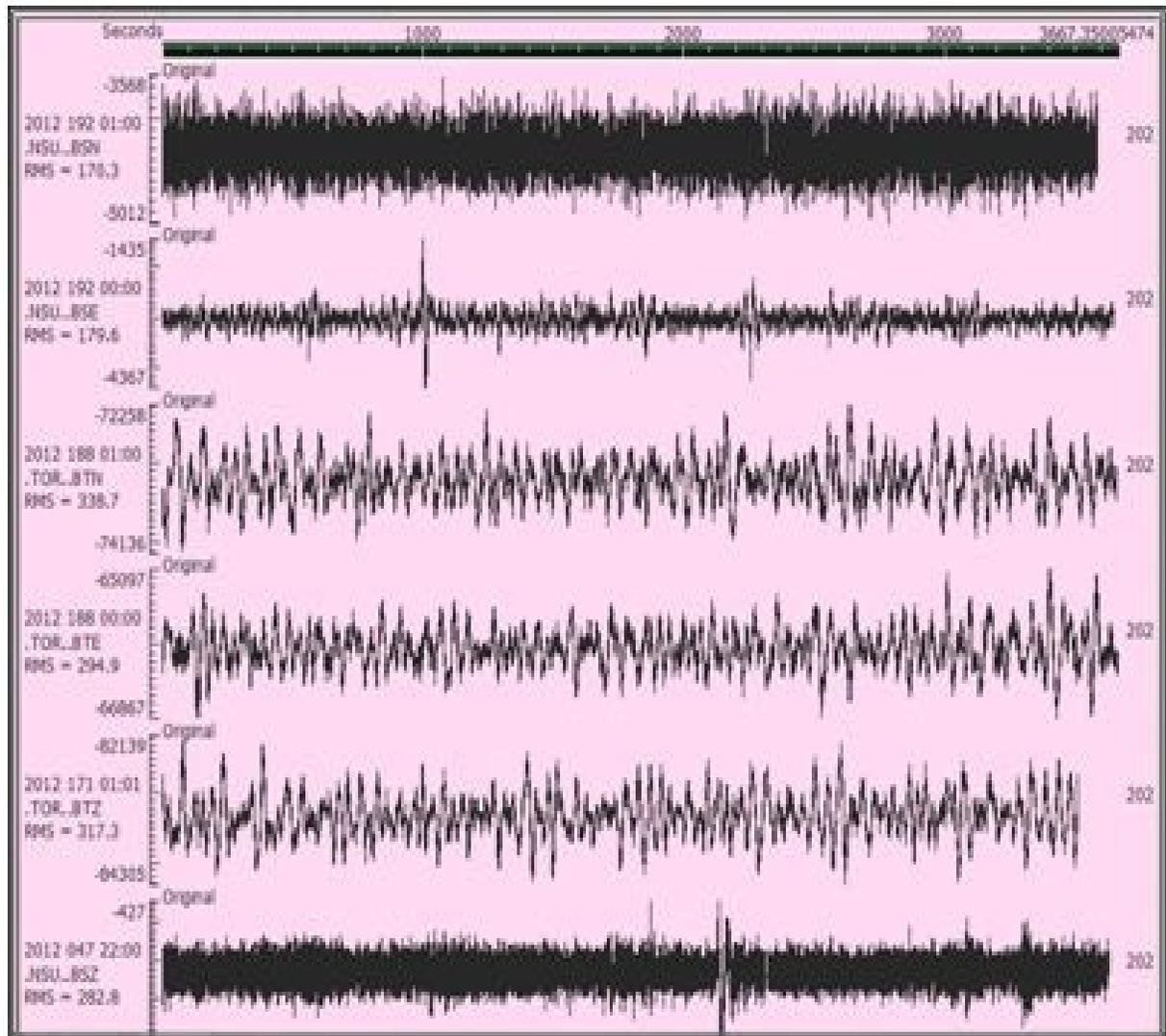
**Figure 7.** Traces of Z, N, E, components from Toro and Nsukka stations. High noise levels are clearly observed on the components of Nsukka station. If for instance there is an event at the time the seismic traces from Nsukka in this figure were recorded, the event will be completely shrouded by noise, thereby compromising quality of the signal. This is not good for signal to noise ratio of a station.
