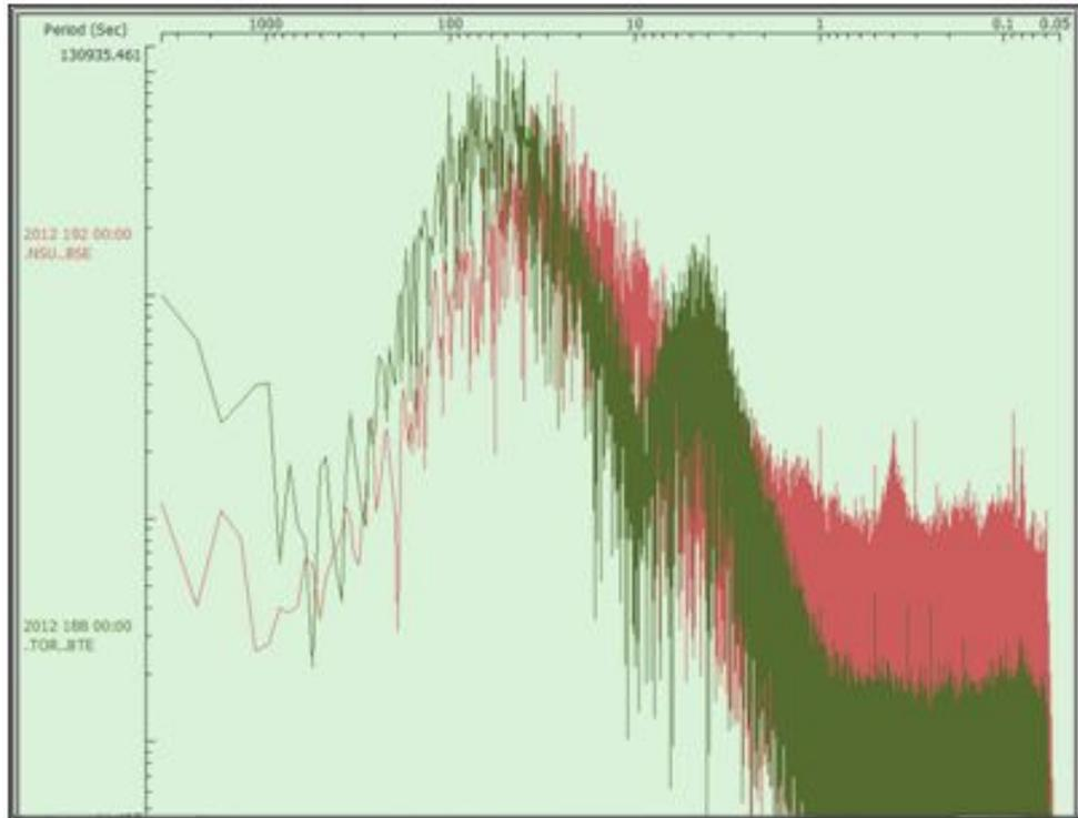
**Figure 10.** Overly of the vertical (Z) component of Toro and Nsukka showing higher noise on the Nsukka component (green colour). The red colour represents trace from Toro.
