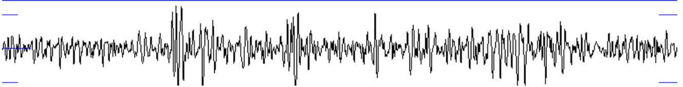
**Figure 4.** Filtered trace from Nsukka (using 0.01 to 0.1Hz filter band), the signal-to-noise ratio is much improved and later phases are clearly recognizable since the microseisms have been removed by filtering (courtesy: Havscov and Ottemoller, 2008).
