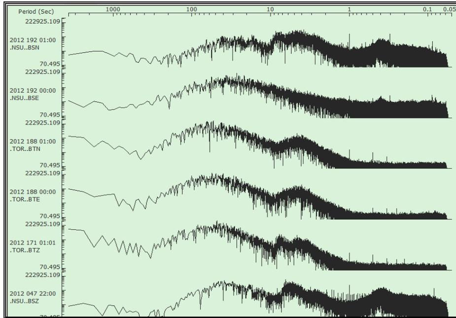
**Figure 8.** Spectral figures from the three components of Toro and Nsukka stations. The spectra from Nsukka station (first, second and sixth in the figure; especially the first and sixth spectra) exhibited high noise at high frequencies compared to the spectra of Toro station (third, fourth and fifth spectra in the figure). It is likely as a result of the contribution of anthropogenic noise from surrounding human activities and natural noise sources like wind.
