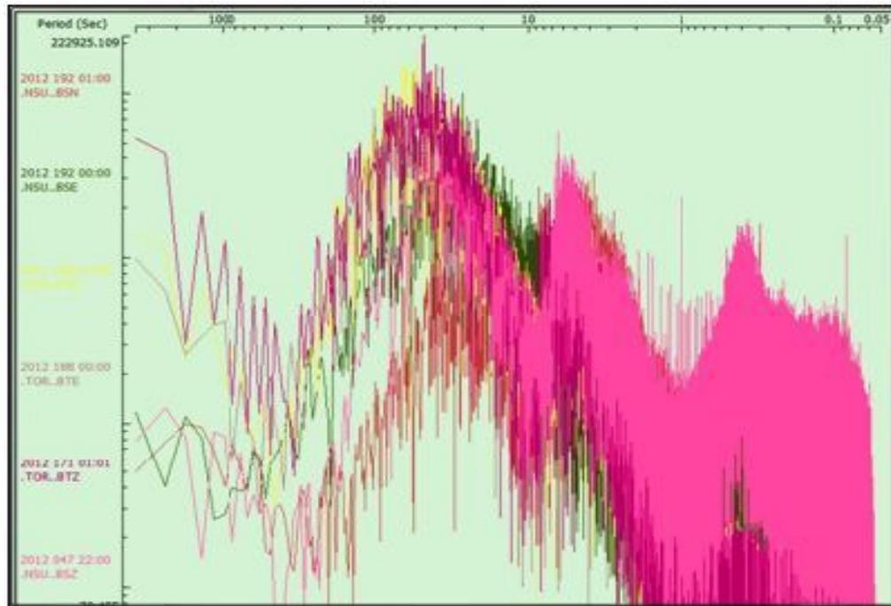
**Figure 12.** Overlay of the three components of Toro with three components of Nsukka showing a remarkable higher noise on the Nsukka component (pink, green and red colours). The yellow, light pink and black colours traces represent Toro station, which are almost covered by the dominance noise from Nsukka.
