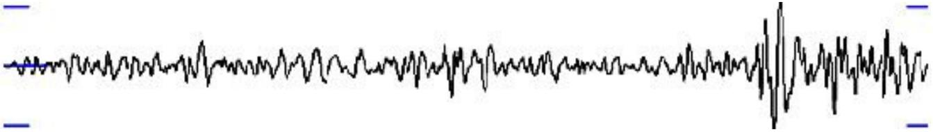
**Figure 6.** Filtered trace using 0.01 to 0.1Hz band-pass of the Toro station. Good SNR at this station does not give room for a distinct difference between Figures 4 and 5, unlike as observed in Figures 2 and 3.
