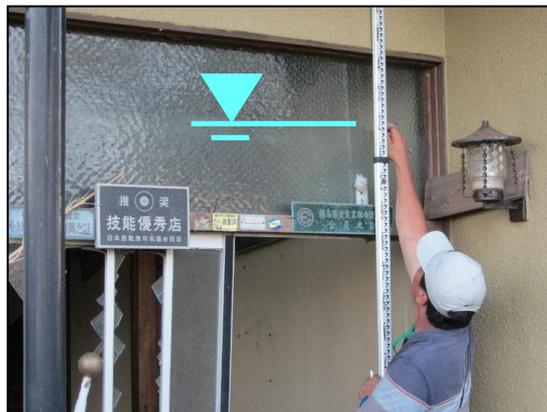
Figure 4. Measurement of tsunami inundation height
