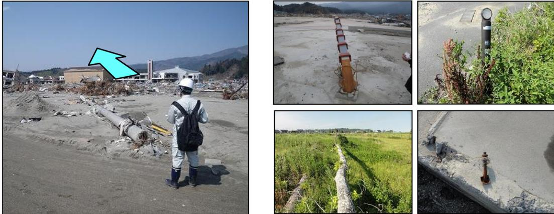
Figure 2. Measurement of tsunami flow direction (left) and examples of pillar-shaped object (right)
