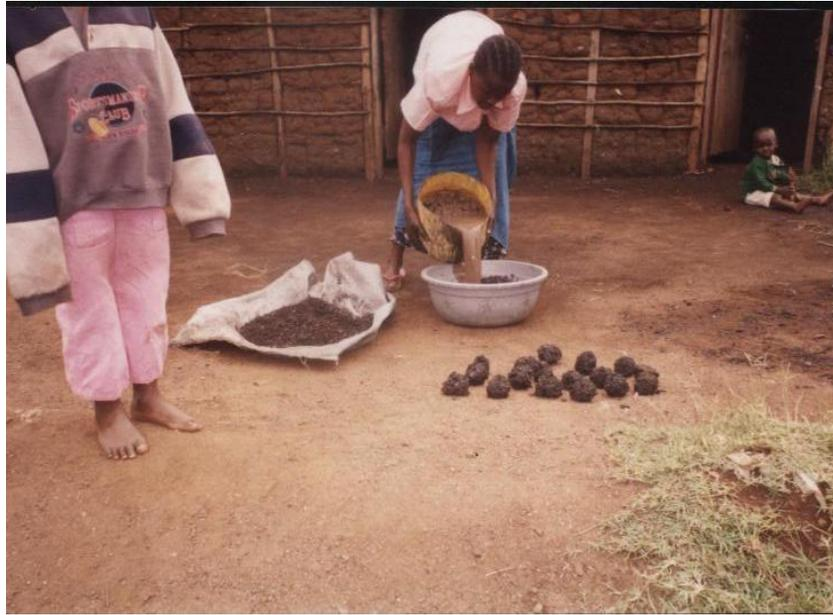
**Figure 5.** Mixing of charcoal fines, clay and water.
