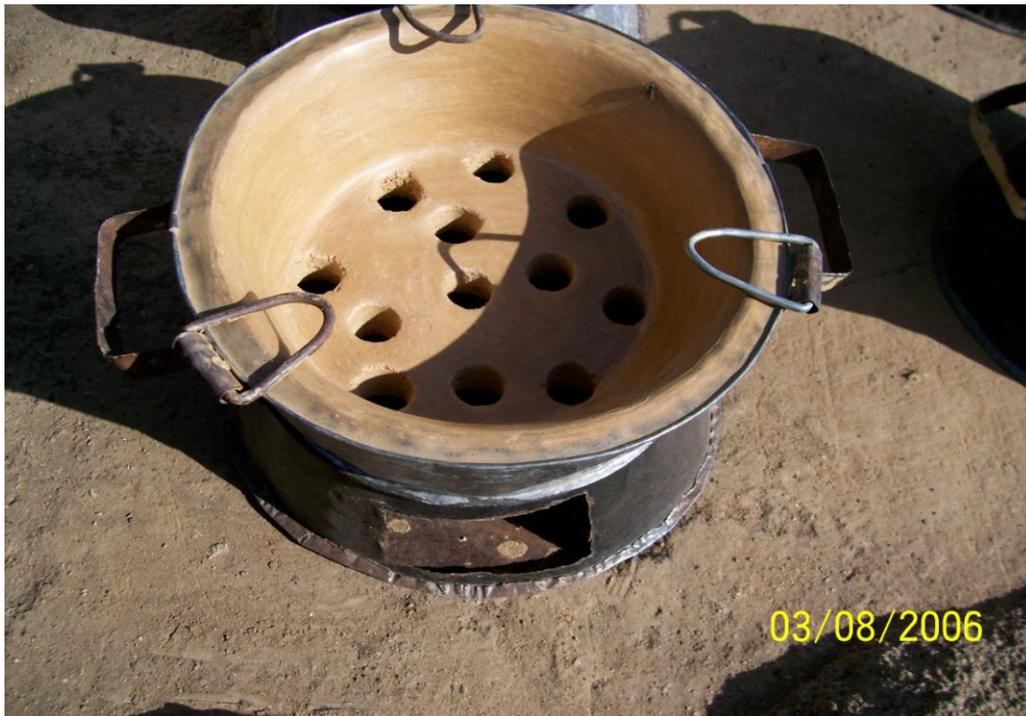
**Figure 4.** The improved stove/upesi jiko with a clay lining and small holes to save energy.
