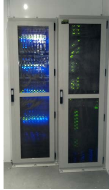
Fig. 5. Front view of LEDA correlator racking (right). Large-format EMI air filters adopted to enable most readily the front-back airflow required by the digital hardware comprise the door. Screening at 40 MHz is \sim 50 \text{ dB} . The left-hand rack contains high-gain analog electronics and is independently shielded against RF interference. RF-tight pass throughs in the common wall convey signals from the analog electronics to the correlator digital samplers. The setup is conceptually similar to that adopted for LWA1 ( Taylor et al., 2012 ; Ellingson et al., 2013 ) though more compact and capable of supporting greater power and computational density.
