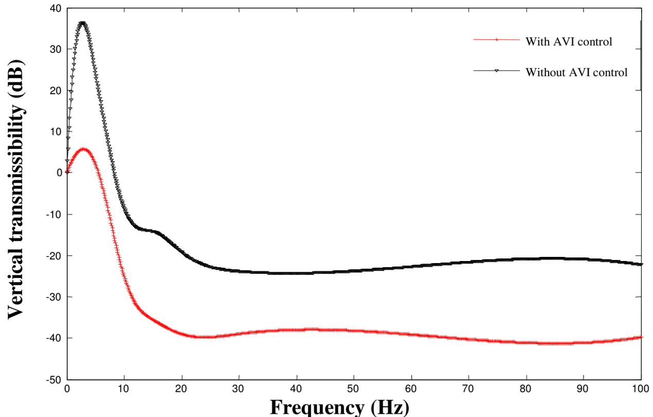
Figure 9. Transmissibility curve with and without AVI control.
