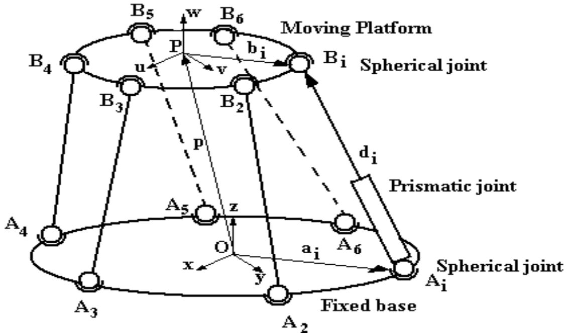
Figure 1. Spatial six DOF, six SPS parallel manipulator.
