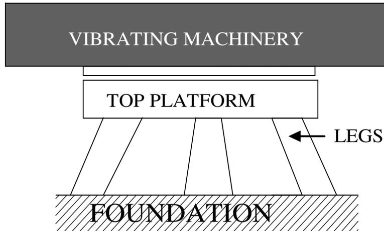
Figure 2. Stewart platform for isolating foundation from machinery vibration.
