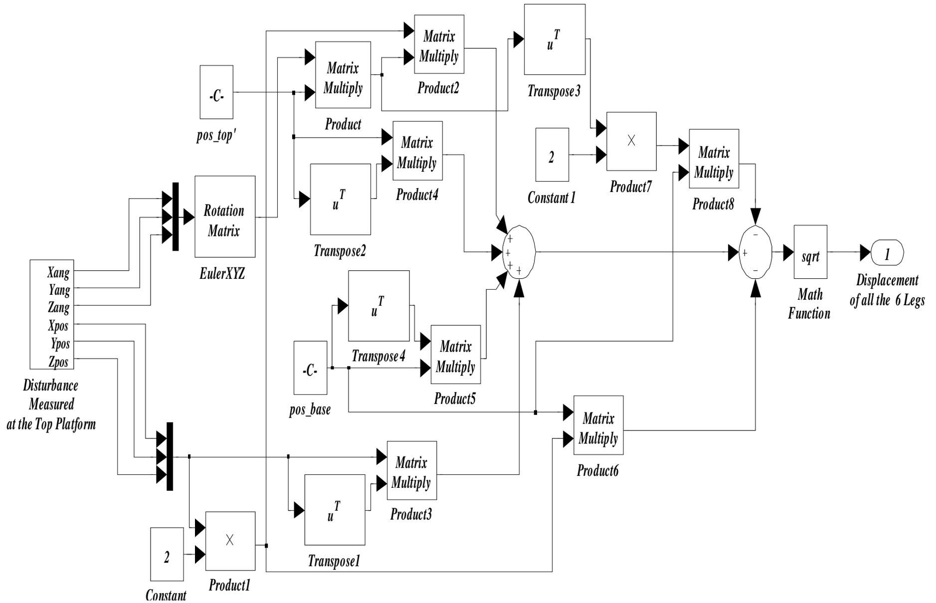
Figure 3. Inverse kinematic equation model in MatLab.
