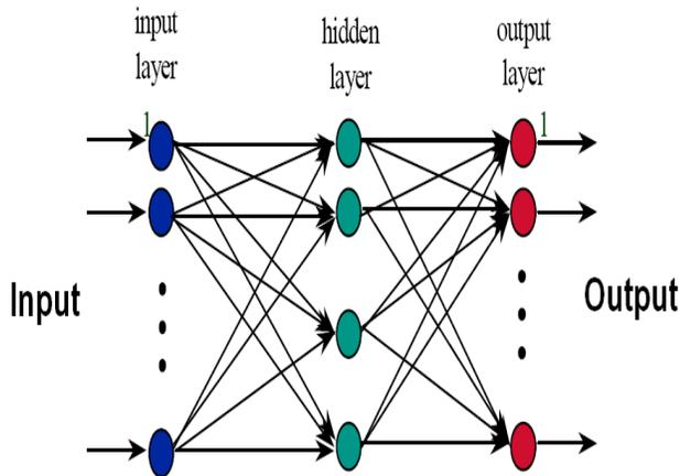
Figure 2. Radial basis function neural networks.
