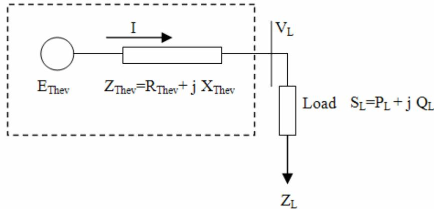
**Figure 1.** A Simple two-bus Thevenin equivalent system.
