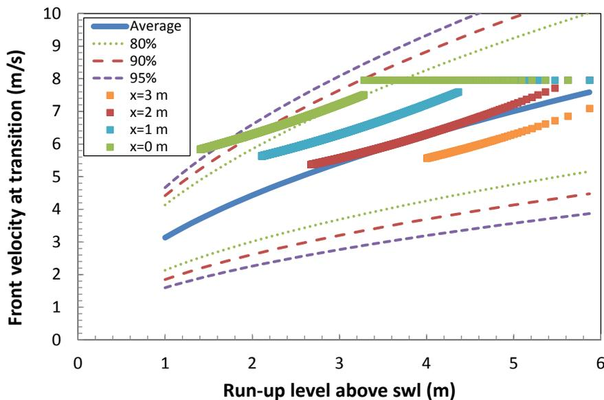
Figure 15. Distribution of front velocities as simulated at the transition from berm to upper slope, compared to the theoretical distribution ( $x$  is the vertical distance from simulated water level to the transition).
