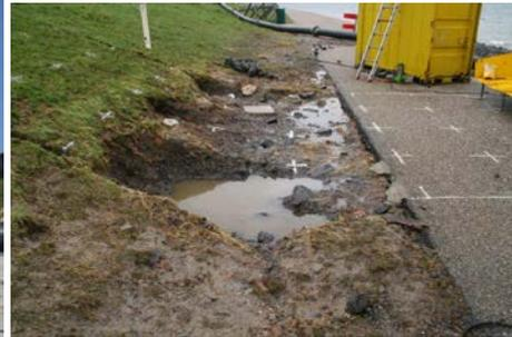
Figure 3. Damage caused by wave run-up simulation.
