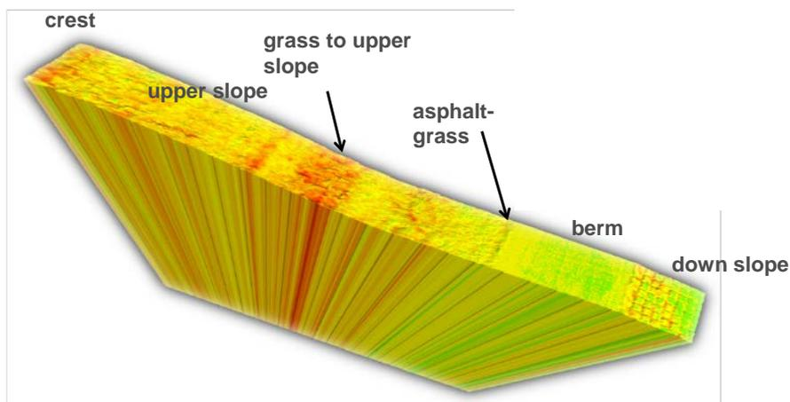
Figure 11. Laser scan of the tested slope of 2 m wide, after test 1. Erosion more than 5 cm is orange to red, no erosion is yellow.
