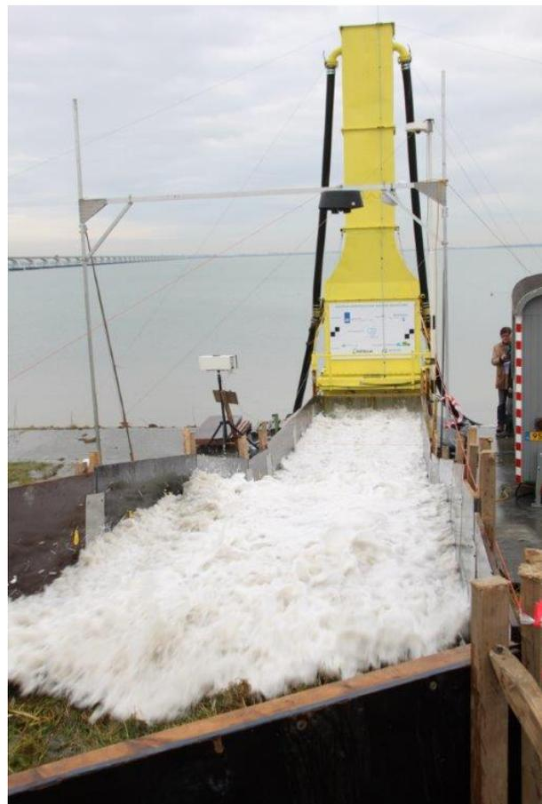
Figure 7. The Wave Run-up Simulator in action
