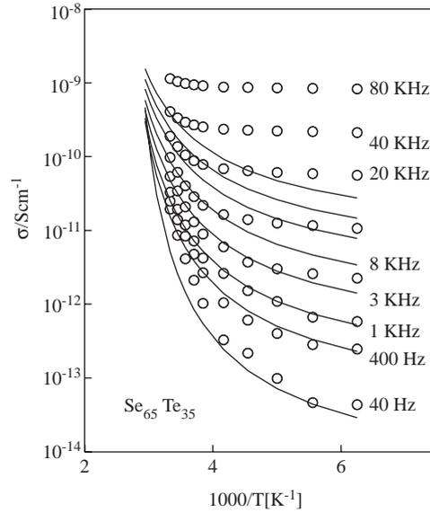
**Figure 2.** AC conductivity of  $\text{Se}_{65}\text{Te}_{35}$  as function of reciprocal temperature for various frequencies.
