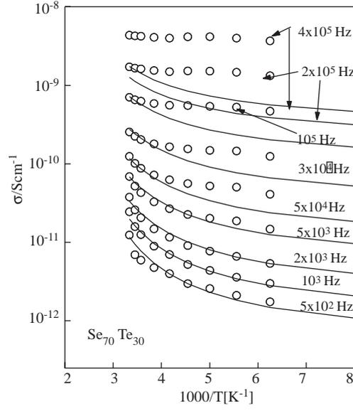
**Figure 1.** The temperature dependences of the measured AC conductivity at various frequencies for  $\text{Se}_{70}\text{Te}_{30}$  thin film. The solid curves are calculated results using Eq. (7).
