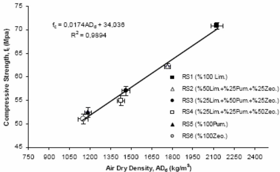
**Figure 4.** The relation between air dry density and compressive strength.
