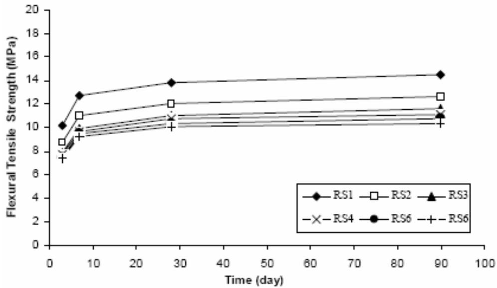
**Figure 3.** Flexural tensile strength of lightweight polymer concrete.
