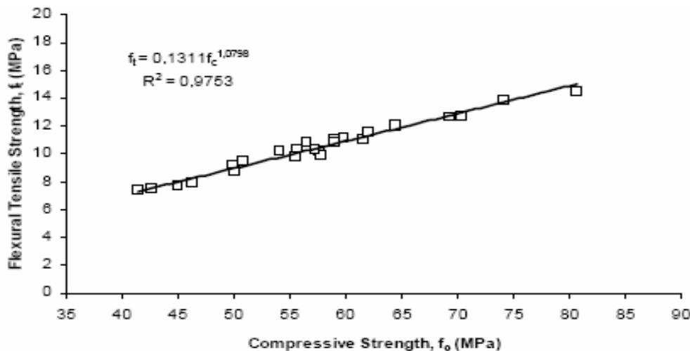
Figure 6. The relation between flexural tensile and compressive strength.
