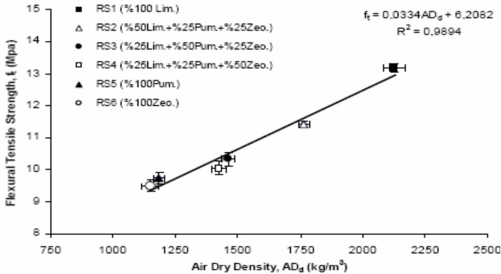
Figure 5. The relation between air dry density and flexural tensile strength.
