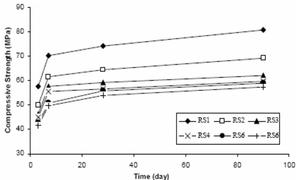
**Figure 2.** Compressive strength of lightweight polymer concrete.
