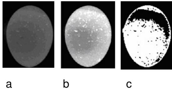
**Figure 7.** Image processing of I (a-Gray scale image, b-Adaptive contrast enhancement, c- Binary image).
