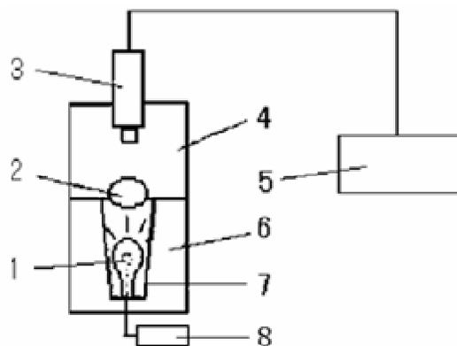
**Figure 1.** Computer vision device of egg image (1-Light source, 2-Egg, 3-Digital camera, 4-Dark room, 5-Computer, 6-Light room with radiator, 7-Light tube, 8-Transformer)
