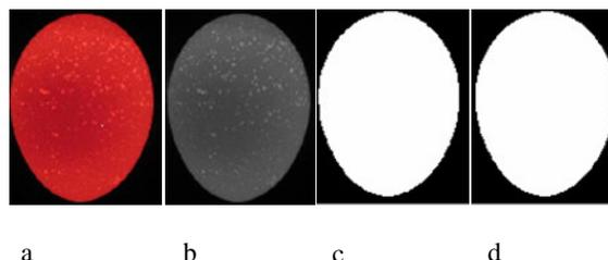
**Figure 2.** Egg image processing (a-Original image, b-Gray scale image, c-Binary image, d-Median filter).
