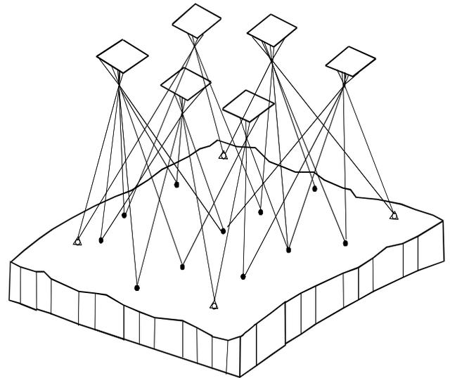
**Figure 2.** Block balancing by bundle adjustment.
