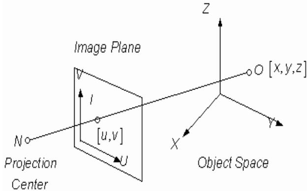
**Figure 3.** General view of picture and object coordinate system.
