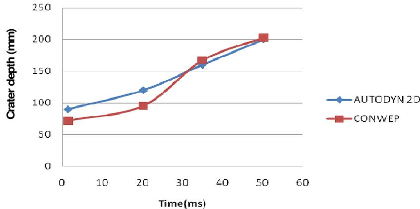
**Figure 9.** Comparison of crater depth and time variations between numerical simulation and experimental findings.
