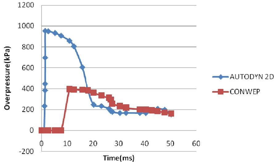
**Figure 7.** Comparison of overpressure and time between numerical simulation and experimental (CONWEB).
