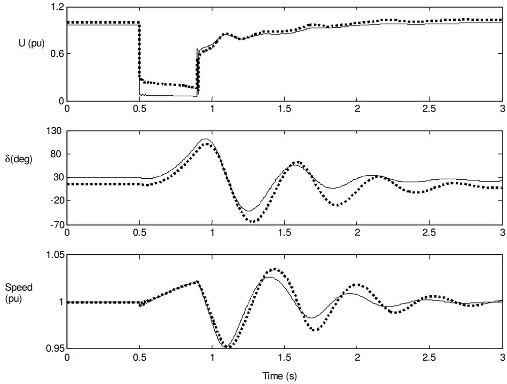
Figure 5. Responses of embedded generators for case 1c, dotted: small unit, solid: big units.
