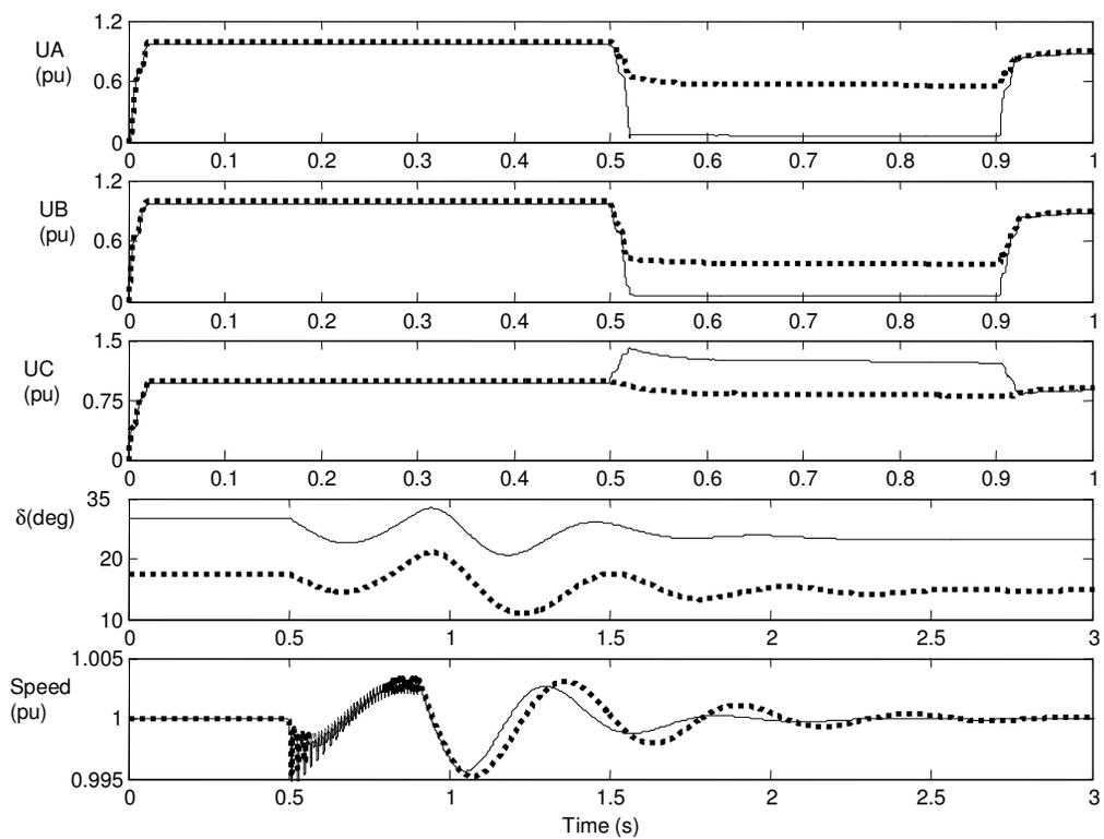
**Figure 10.** Responses of embedded generators for case 3b, dotted: small unit, solid: big units.
