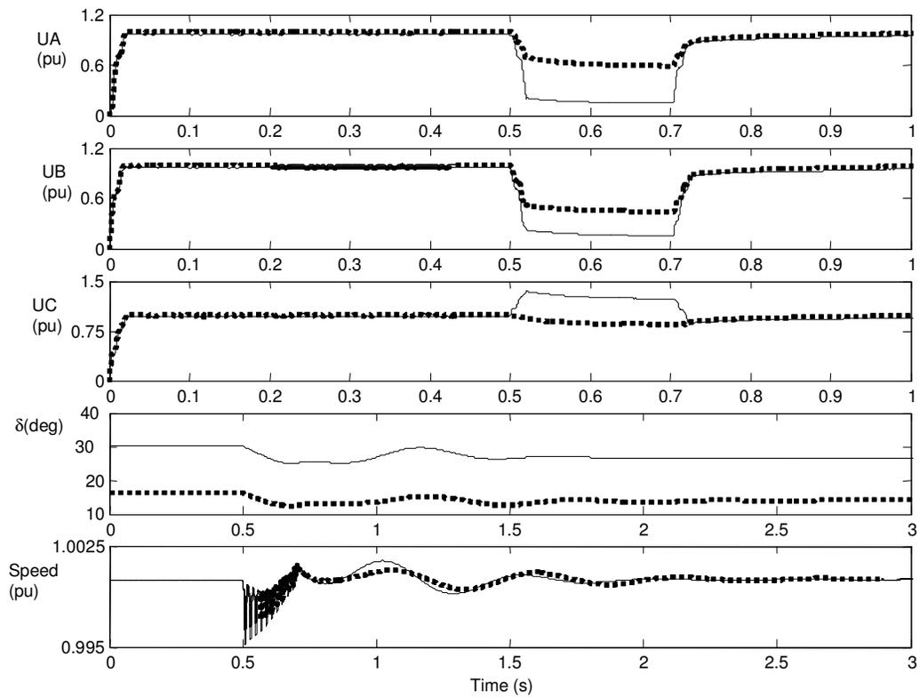
**Figure 9.** Responses of embedded generators for case 3a, dotted: small unit, solid: big units.
