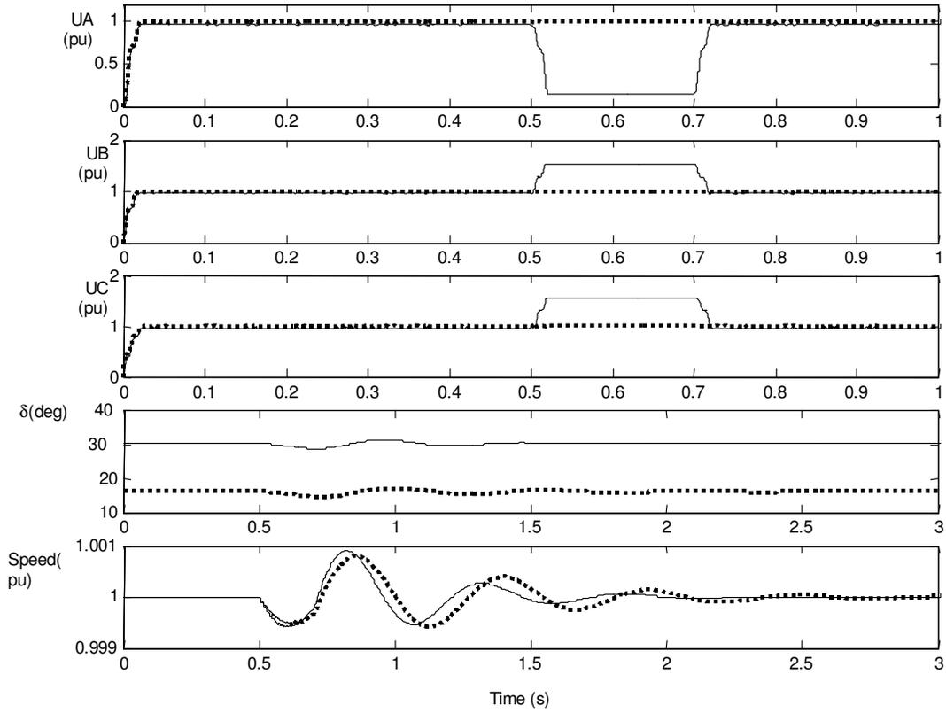
Figure 7. Responses of embedded generators for case 2a, dotted: small unit, solid: big units.
