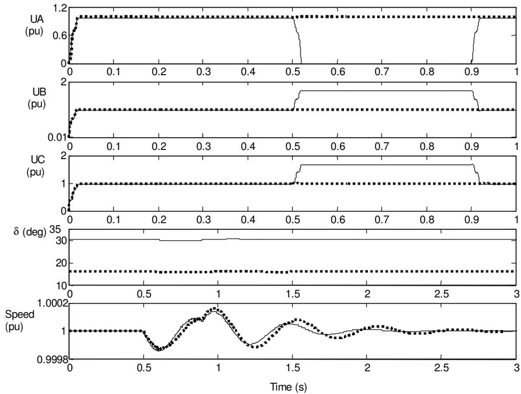
Figure 8. Responses of embedded generators for case 2b, dotted: small unit, solid: big units.
