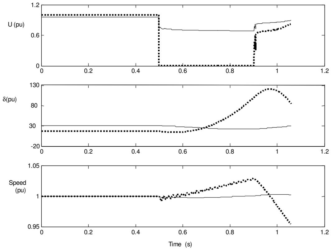
Figure 6. Responses of embedded generators for case 1d, dotted: small unit, solid: big units.
