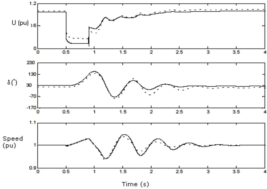
**Figure 3.** Responses of embedded generators for case 1a, dotted: small unit, solid: big units.
