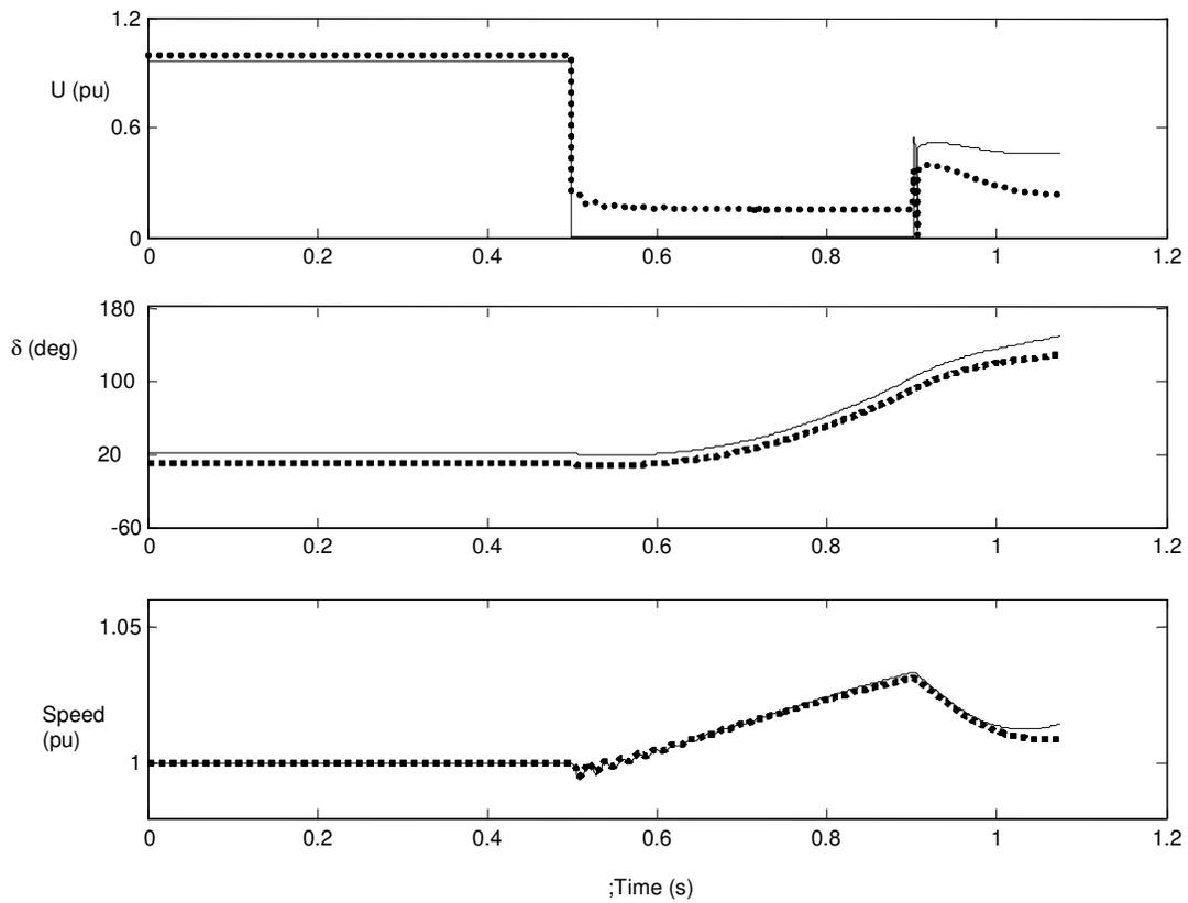
**Figure 4.** Responses of embedded generators for case 1b, dotted: small unit, solid: big units.
