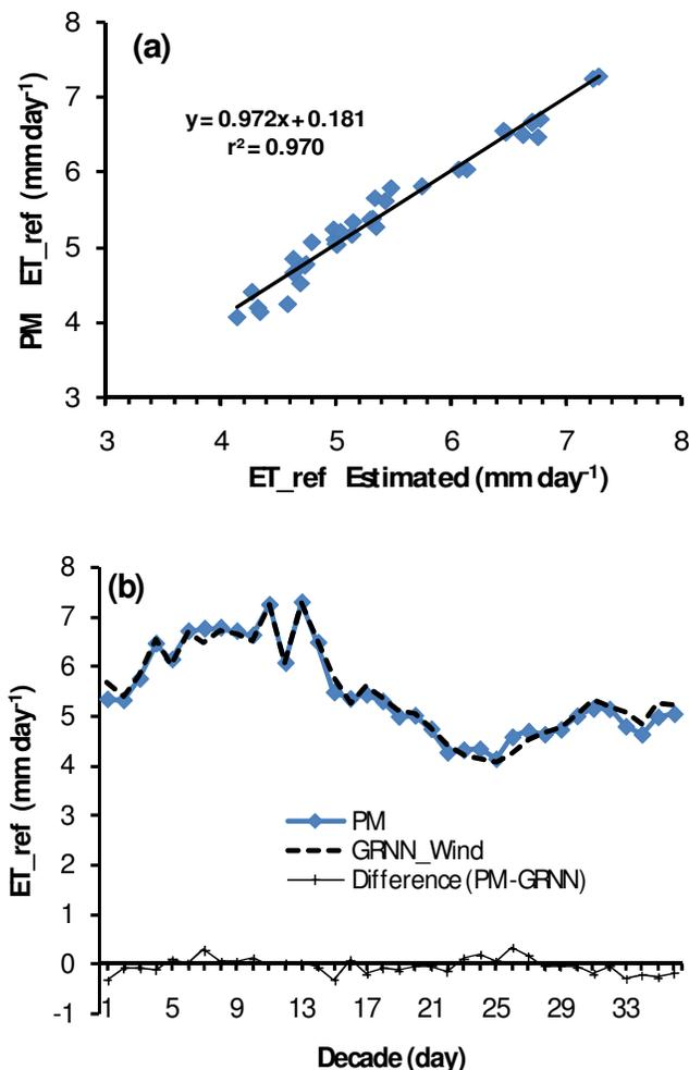
**Figure 4.** GRNN scatter (a) and plot (b) during the testing period when wind speed is integrated into the neural network model.
