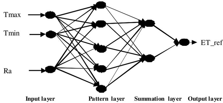
Figure 2. Schematic diagram of GRNN architecture.
