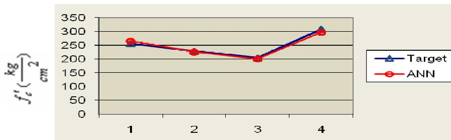
Figure 8. Evaluation of target and predicted compressive strength by ANN.
