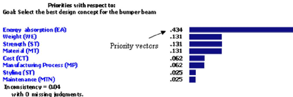
Figure 9. The priority vectors and consistency test for the main criteria with respect to the goal.
