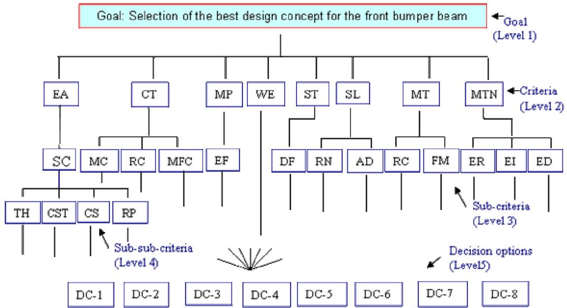
**Figure 7.** The hierarchy model (4 levels) represents the criteria and sub-criteria affecting the selection of design concepts for automotive bumper beam.
