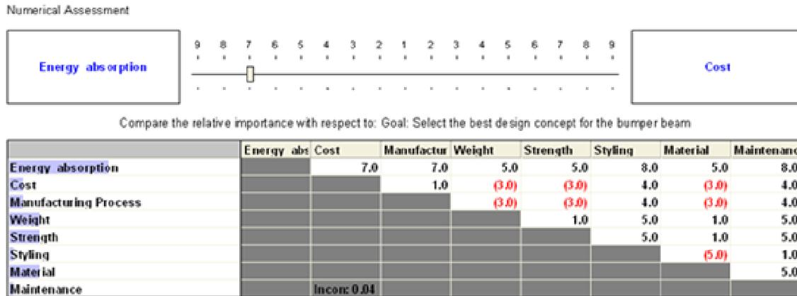
Figure 8. Pair-wise comparison of the main criteria with respect to the goal in a matrix format as a result of using Expert Choice software.
