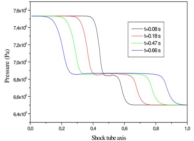
**Figure 6.** Pressure profiles along the shock tube for different time steps.
