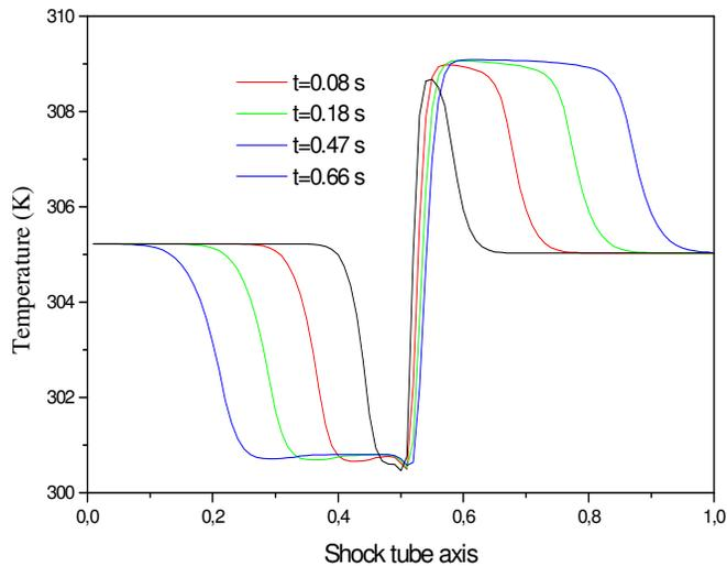
**Figure 4-** Temperature profiles along the shock tube for different time steps.
