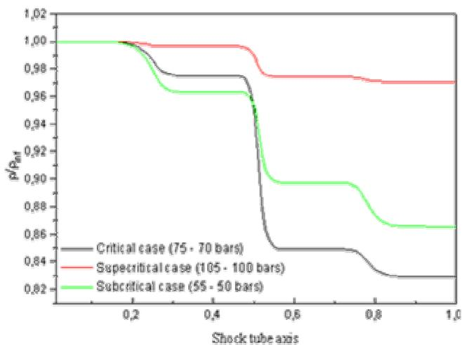
Figure 8. Dimensionless density profiles along the shock tube for different expansion ratios (effect of the critical region behaviour)
