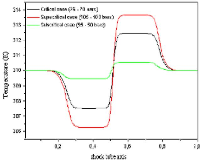
Figure 7. Temperature profiles along the shock tube for different expansion ratios (effect of the critical region behaviour).
