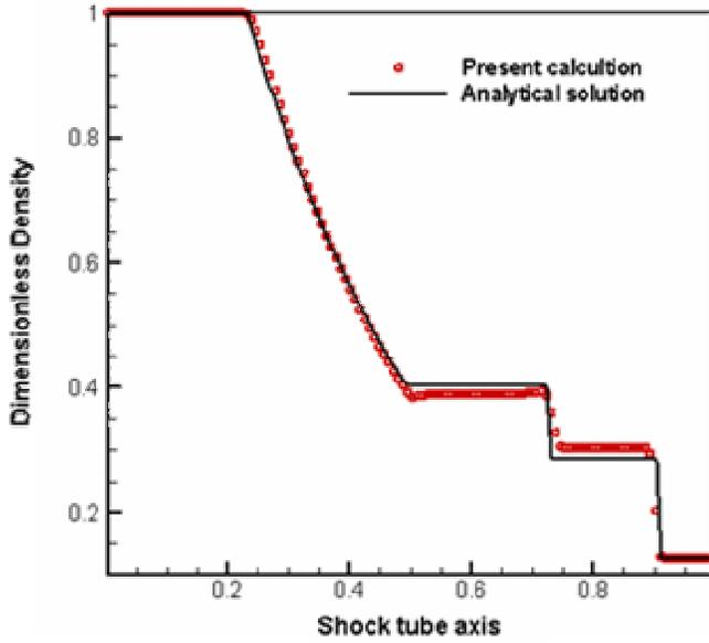
**Figure 2-** Numerical validation of the shock tube problem for sub-critical conditions, at a dimensionless time  $t = 0.2$  s
