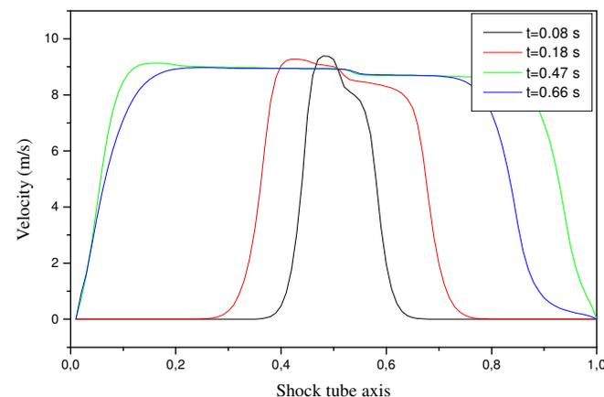
**Figure 5.** Velocity profiles along the shock tube for different time steps.
