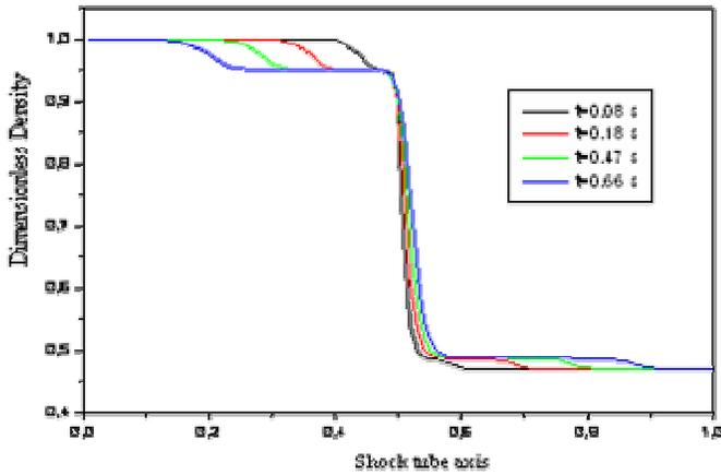
**Figure 3-** Dimensionless density profiles along the shock tube for different time steps.
