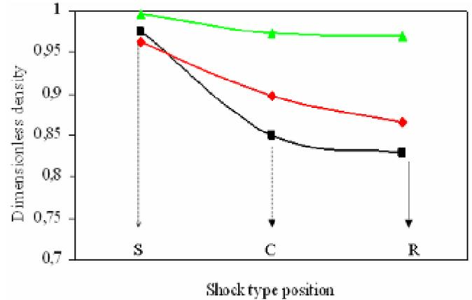
Figure 9. Density falls under the action of the various shock waves (S, C, R).
