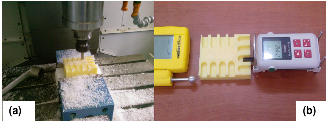
Figure 1. The pictures of experiment setting. (a) CNC machining (b) Surface roughness measurement.
