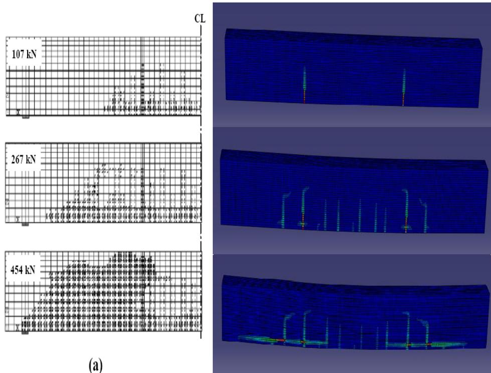
Figure 12. Crack patterns in process of analysis.
