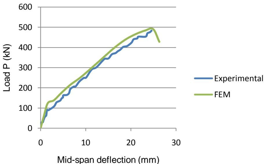
Figure 11. Load-deflection plot for the beam.
