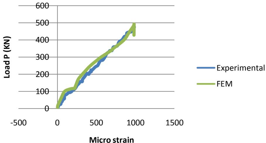
Figure 10. Load-compressive strain plot for concrete.
