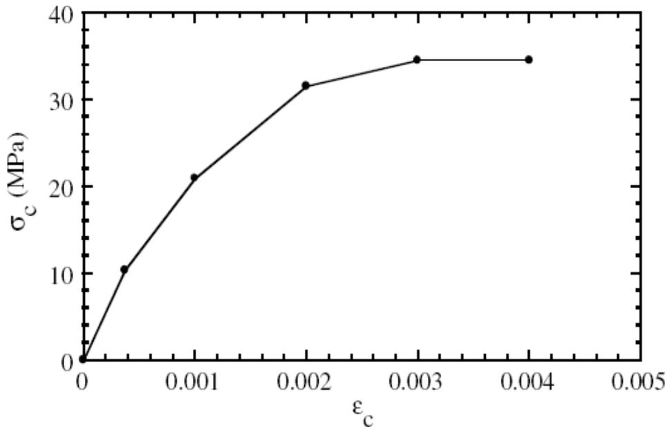
Figure 6. Equivalent uniaxial stress-strain curve for concrete.
