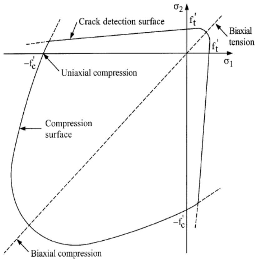
Figure 5. Concrete failure surface in plane stress.
