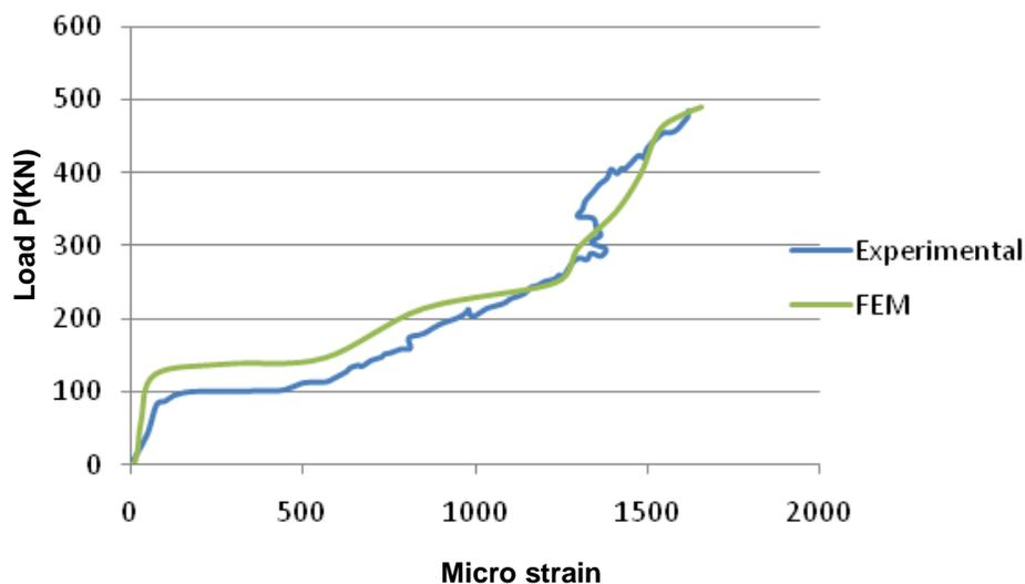
Figure 9. Load-tensile strain plot for main steel rebar.
