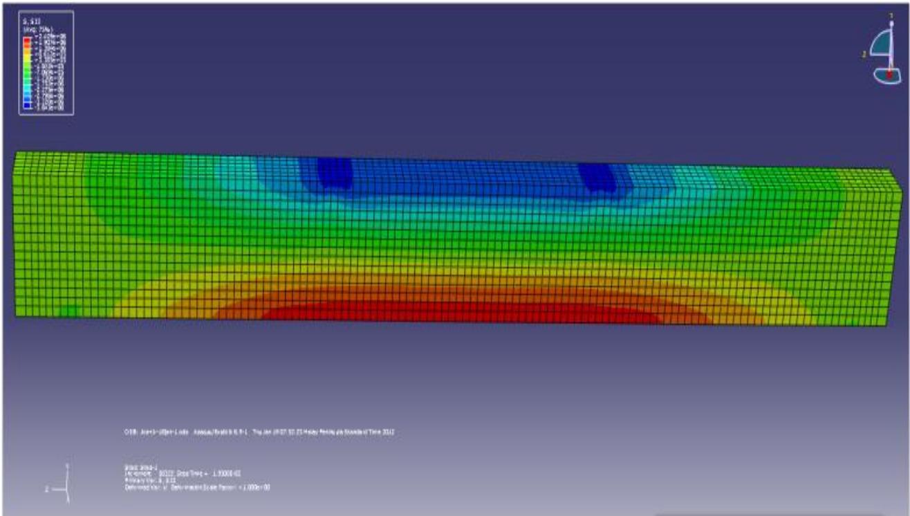
Figure 4. Concrete stresses.
