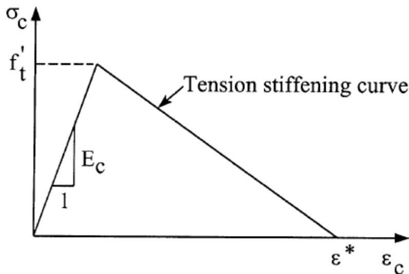
Figure 7. Tension stiffening model.
