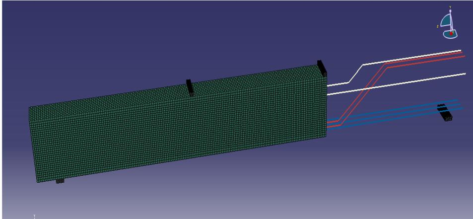
Figure 8. Concrete meshed model in ABAQUS.
