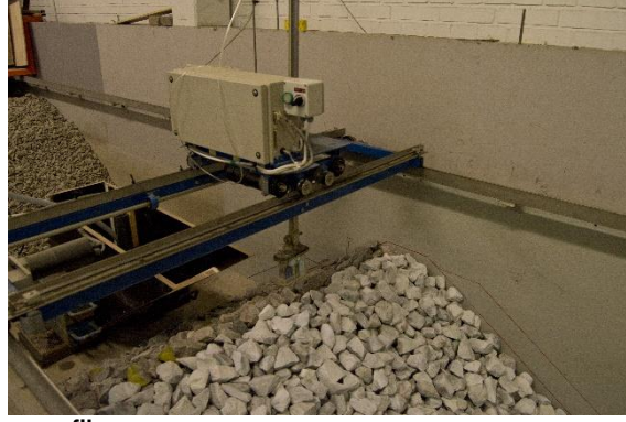
Figure 5: Set-up of erosion profiler.
