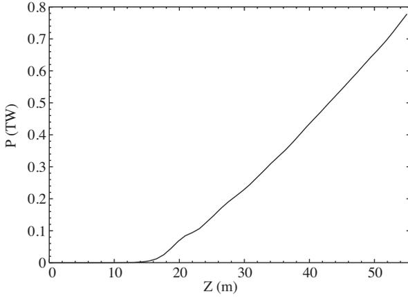
**Figure 4.** FEL Power as a function of wiggler length.
