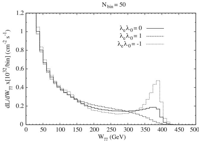
**Figure 2.** CLIC  $\gamma\gamma$  Luminosity spectra at  $E_{cm} = 0.5$  TeV for different helicity states of electron ( $\lambda_e$ ) and FEL photons ( $\lambda_0$ ).
