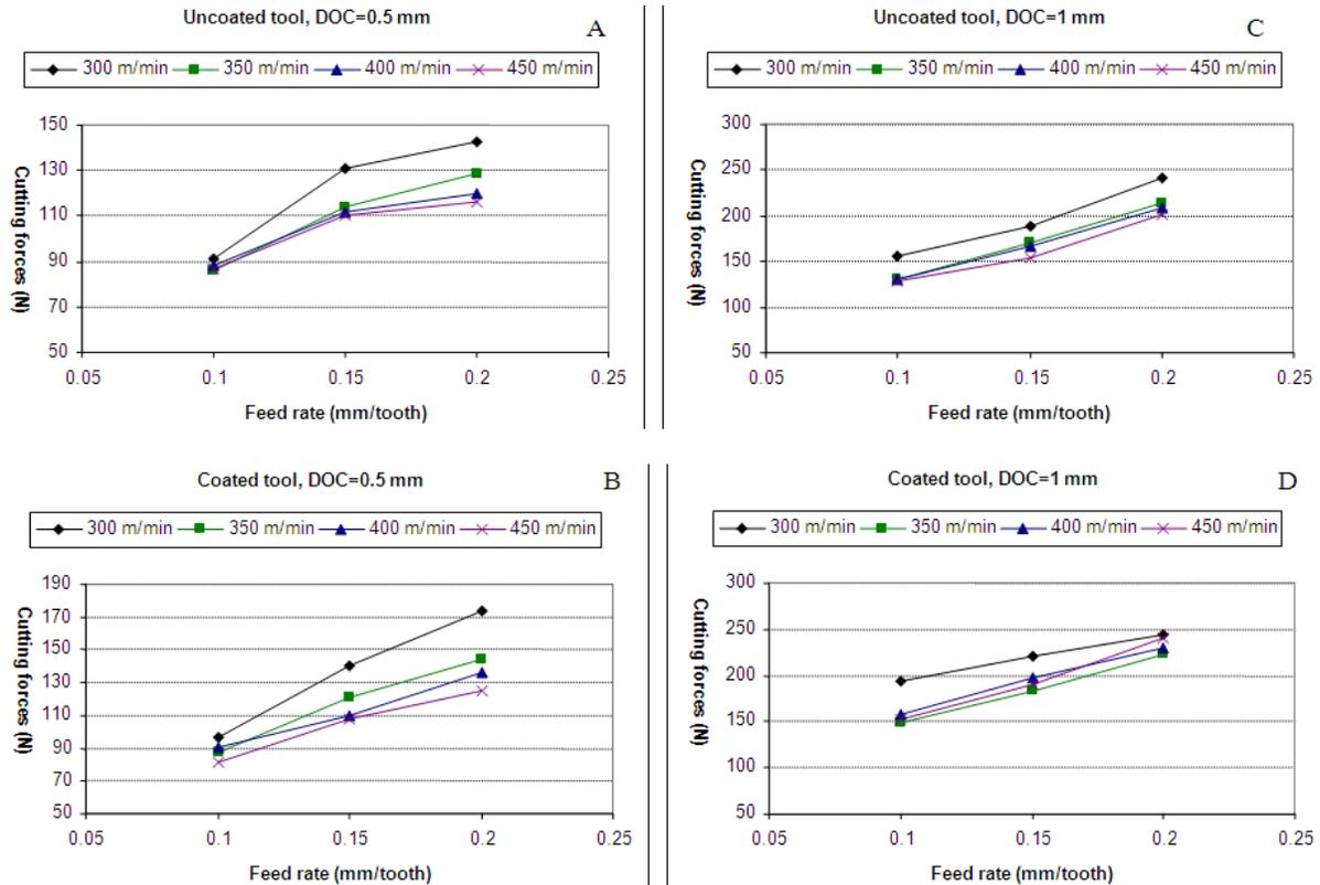
**Figure 3.** Change in main cutting force with respect to the feed rate.
