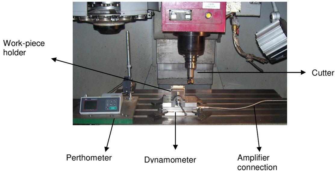
Figure 1. General view of the experimental set-up.
