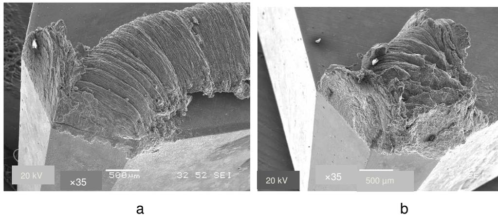
**Figure 6.** Built-up edge formation on the coated tool a) cutting speed of 400 m/min, feed rate = 0.1 mm/tooth and DOC= 1mm, b) cutting speed of 400 m/min, feed rate = 0.2 mm/tooth and DOC= 1 mm ( $\times 35$ ).
