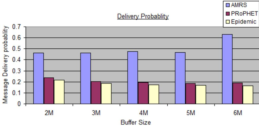
Figure 10. Delivery probability by varying buffer size.
