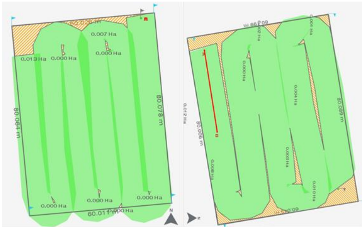
Figure 7. Missed area in fertilizer spreader for Field No. 1 (a) Without navigator (b) With navigaor.
