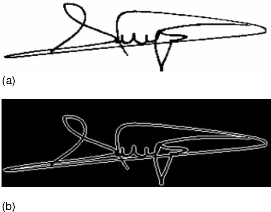
**Figure 4.** A signature before and after edge detection operation. (a) A signature before edge detection; (b) A signature after edge detection.
