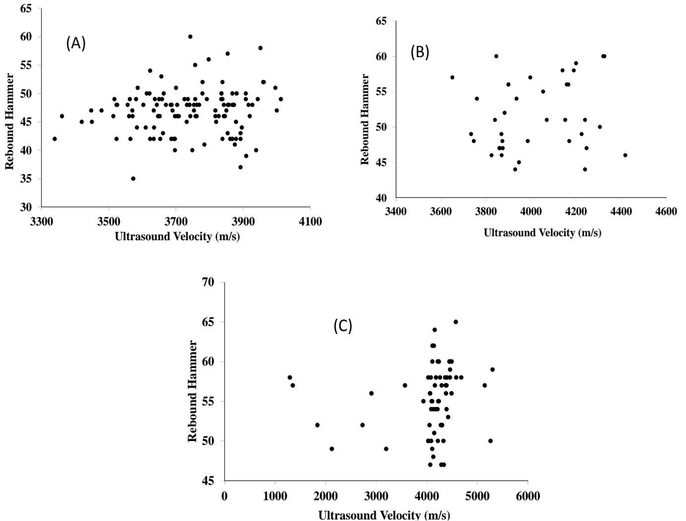
**Figure 8.** Scatter plots of the means obtained using ultrasound and rebound hammer measurements at the three bridges: bridge 1 (a); bridge 2 (b) and bridge 3 (c).
