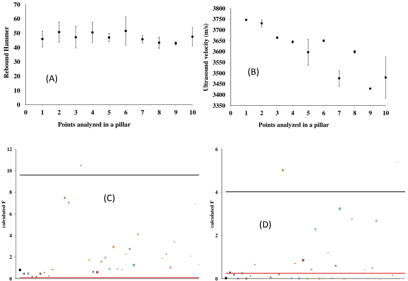
**Figure 7.** Measurements at a pillar of Bridge 3 for the method 2. a) Rebound Impact; b) Ultrasound; Application of the F-test to the impact (c) and ultrasound (d) data; Legend is available in the Figure 5 e).
