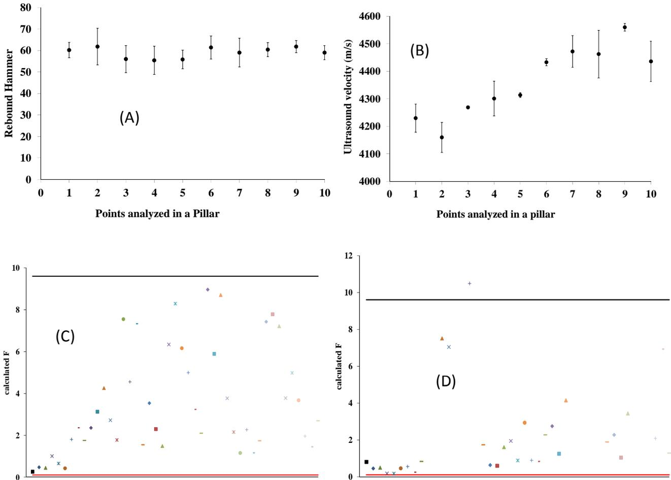
**Figure 6.** Measurements at a pillar of Bridge 2 for the method 2. a) Rebound Impact; b) Ultrasound; Application of the F-test to the impact (c) and ultrasound (d) data; Legend is available in the Figure 5(e).
