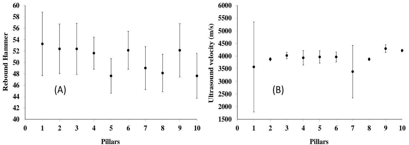
Figure 4. Mean values and confidence intervals with application of the Student's t-test using data from the method (1) at Bridge 1: (a) Rebound impact; (b) Ultrasound.
