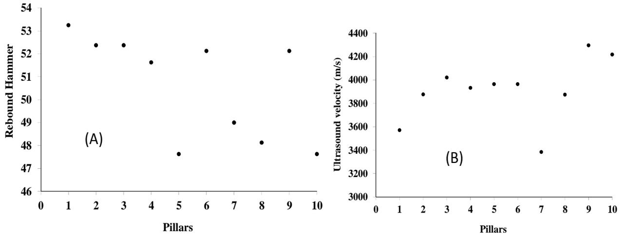
Figure 3. Mean values using data from the method (1) at Bridge 1: (a) Rebound impact; (b) Ultrasound.
