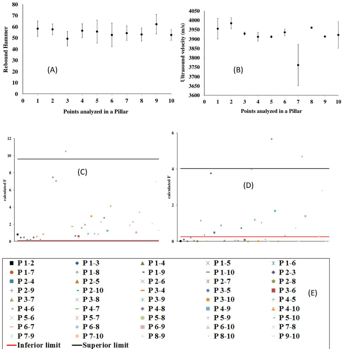
**Figure 5.** Measurements at a pillar of Bridge 1 for the method 2. a) Rebound Impact; b) Ultrasound; Application of the F-test to the impact (c) and ultrasound (d) data; e) Legend to Figures 5 to 7, relating to items (c) and (d), where the P-X-Y notation means the value of the pillar  $F_{calculated}$
