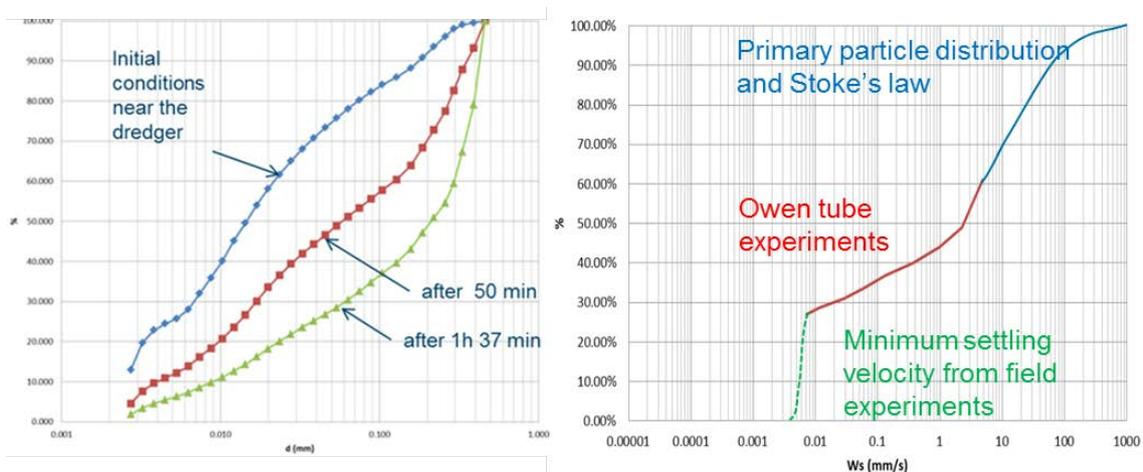
Figure 7. Left: measured grain size distribution in the plume from a trial dredging. Right: example of distribution of settling velocities based on primary particle sizes, experiments in Owen types and measurements in the field.
