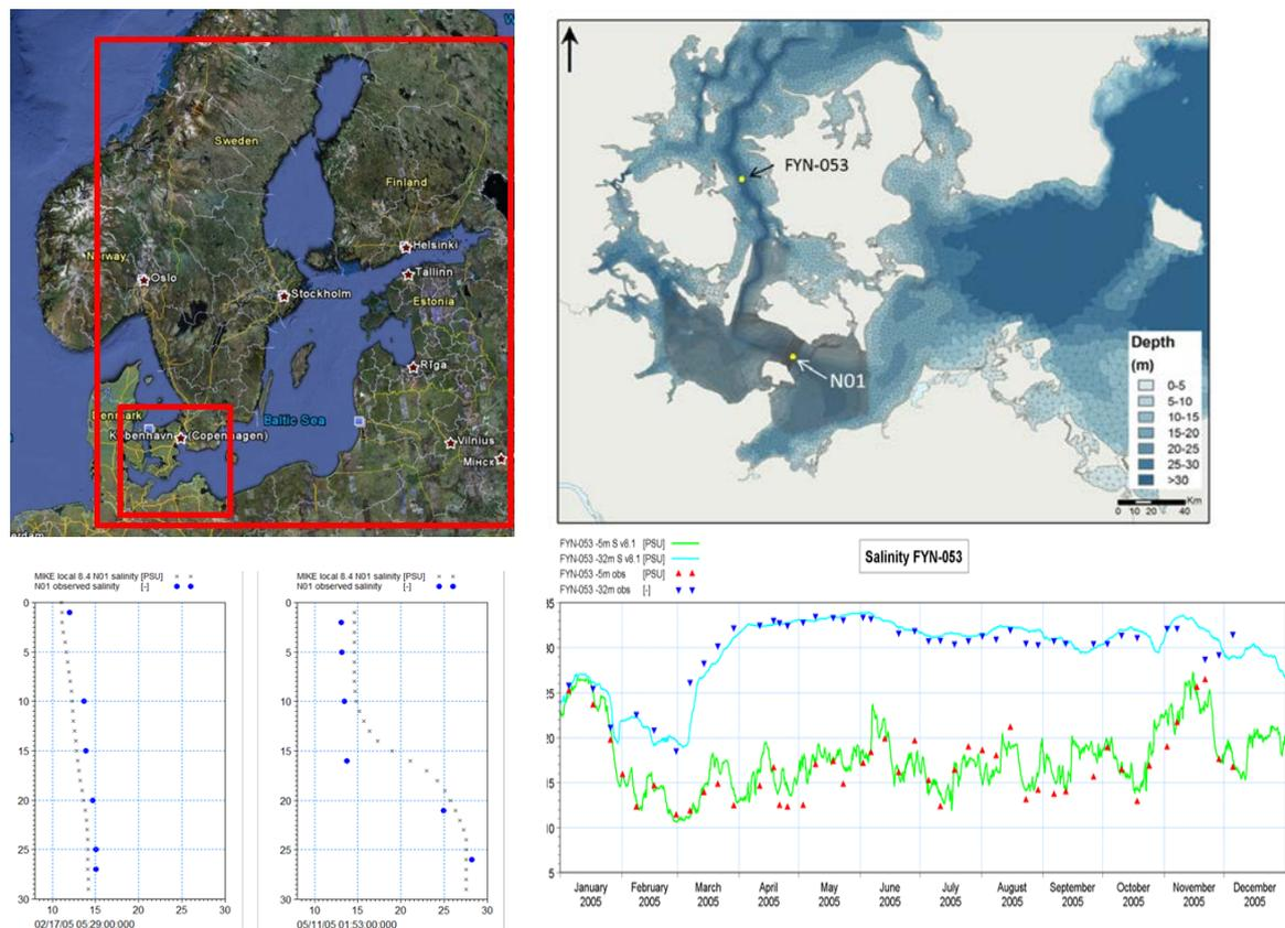
Figure 5. Upper left: the extent of the regional hydrodynamic model. Upper left: the local numerical model area showing computational mesh. Lower left: comparison of measured and modelled salinity at the station M01 at a point in time with no stratification and one with stratification. Lower right: comparison of measured and modelled salinity near surface and bottom at the station FYN-53.
