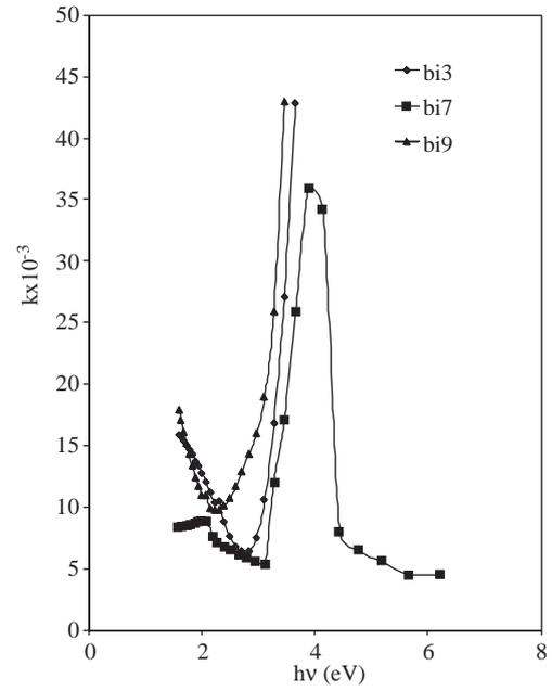
**Figure 8.** Extinction ( $k$ ) as function of photon energy ( $h\nu$ ) for BiOI thin film at 300 K.
