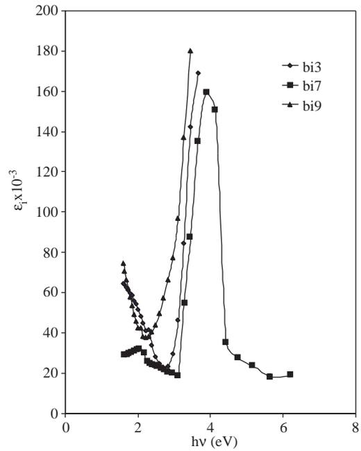
**Figure 10.** Imaginary Dielectric ( $\epsilon_i$ ) as function of photon energy ( $h\nu$ ) for BiOI thin film at 300 K.
