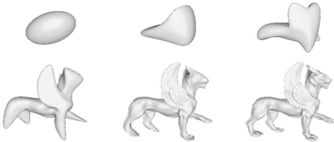
Figure 5. An object constructed using a successive calculation of the frequency components using our approach. The number of calculated frequency components for each version is 2, 8, 14, 45, 64 and 96 respectively.
