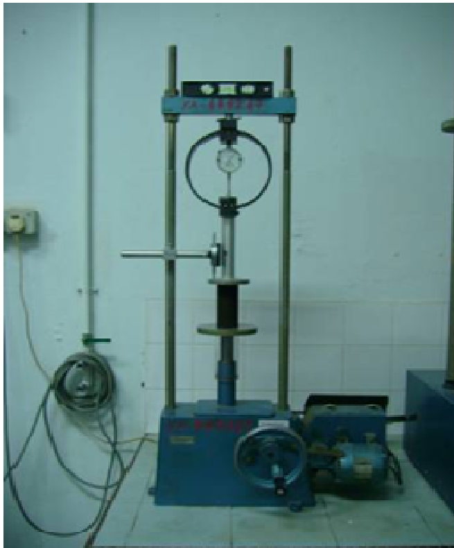
Figure 1. Unconfined compression test using 4.5 kN load frame.
