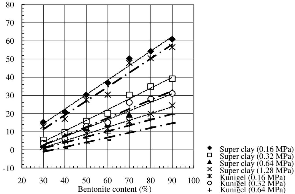
Figure 5. Relationship between maximum percent swelling and bentonite content under static load.
