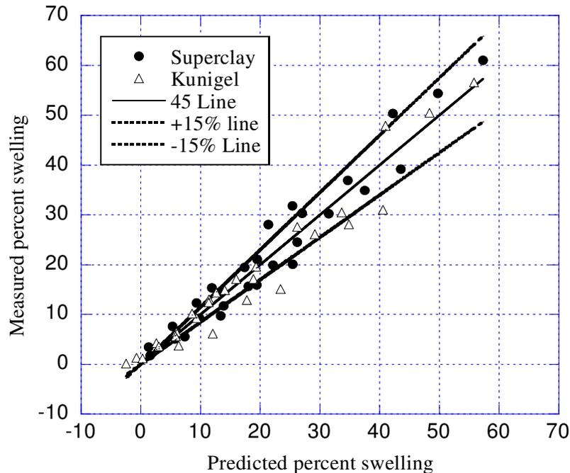
**Figure 6.** Comparison of measure / predicted percent swelling of different content of bentonite in bentonite–sand mixture.
