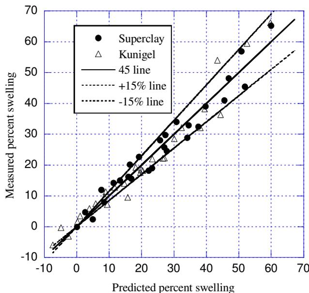
**Figure 4.** Comparison of measured / predicted percent swelling of different densities of compacted solely bentonite.
