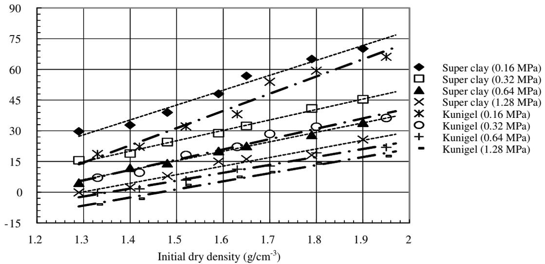
**Figure 3.** Relationship between maximum percent swelling and initial dry density of bentonite under static load.
