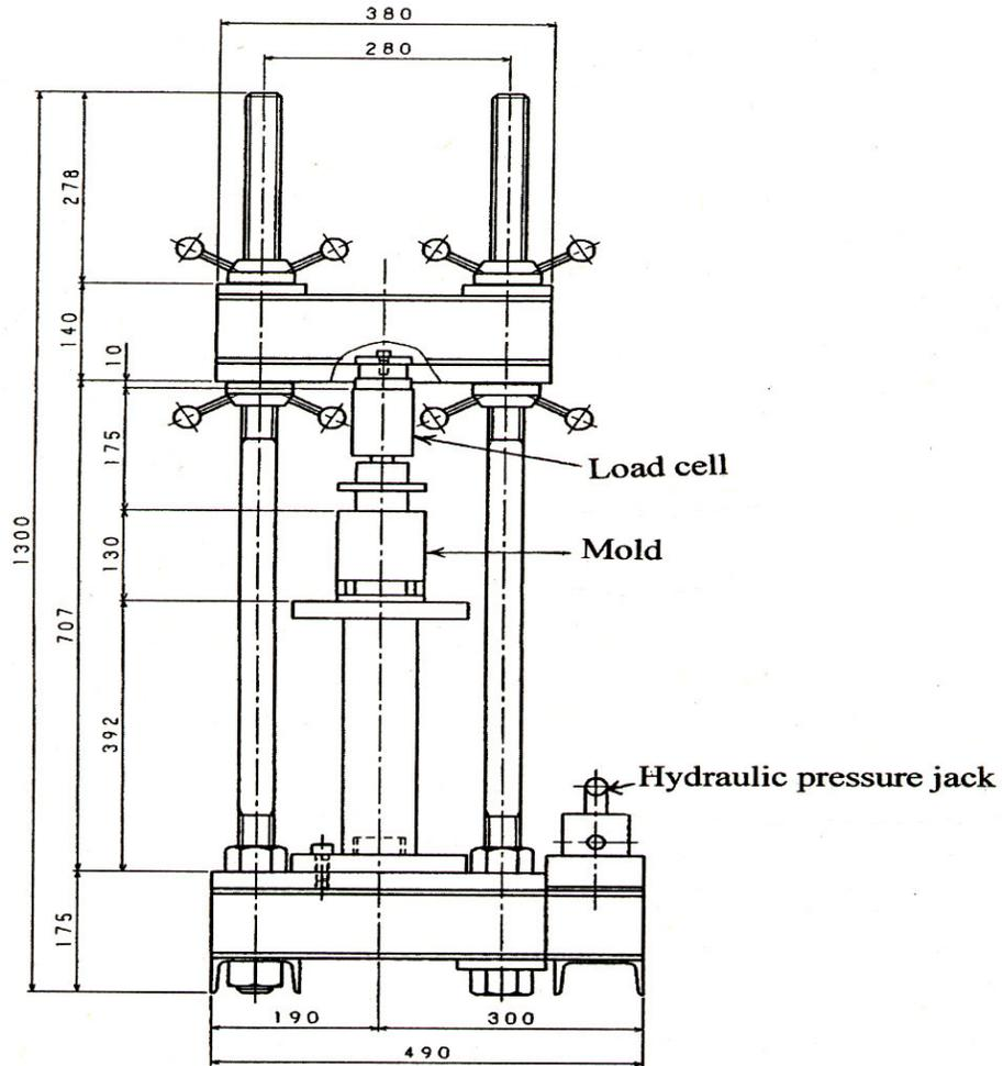
**Figure 2.** Schematic diagram of sample compaction apparatus (Model No. CLP-200KNB). All dimensions are in mm.
