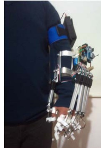
Figure 20. Testing of the hand exoskeleton
