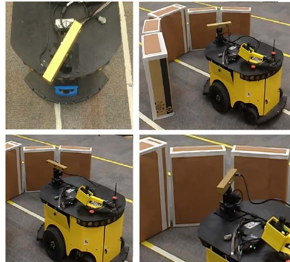
Figure 15. Stereovision based mapping and path planning module capturing observations at different poses
