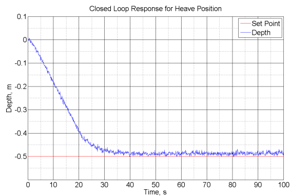
Figure 16. Simulated Response for the Sliding Mode Controller with Thrust Forces of 67 mN and -39 mN
