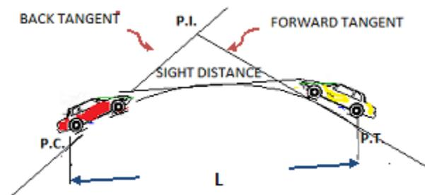
**Fig. 2.** Sight Distance on Vertical Curve.
