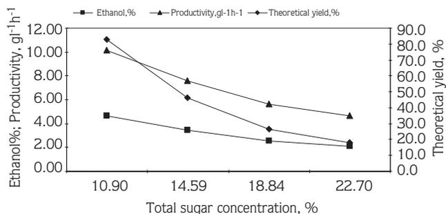
Figure 3. The effect of initial sugar concentration on ethanol production from beet molasses by immobilized yeast cells in a packed-bed bioreactor.
