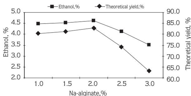
Figure 2. The effect of Na-alginate concentration on ethanol production from beet molasses by immobilized yeast cells in a packed-bed bioreactor ( $T=30^{\circ}\text{C}$ ,  $\text{pH}=3.9$ , initial substrate concentration=10.90%)
