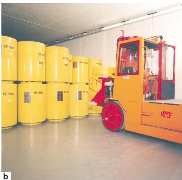
**Figure 5.** (a) Containers for non-heat generating waste, (b) Shielded drums for non-heat generating waste.
