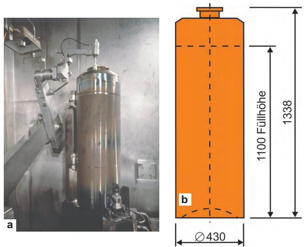
**Figure 4.** Cocilles for vitrified waste and structural parts.
