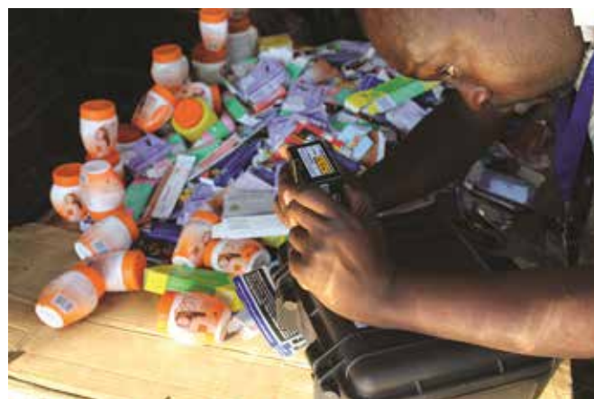
Fig. 4 - Medicines Control Authority Zimbabwe (MCAZ) official testing medicines at a street stall using a Raman spectrophotometer.
