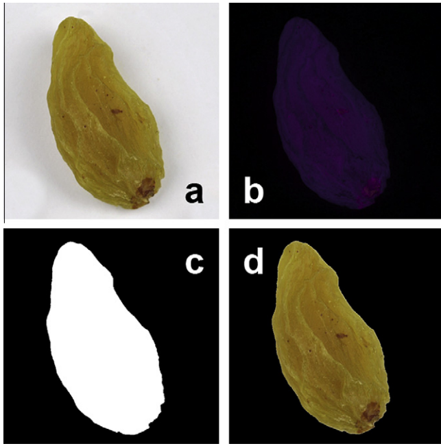
Fig. 3. Image pre-processing: (a) original RGB image, (b) image after being subtracted from background image, (c) binary image, and (d) segmented image.
