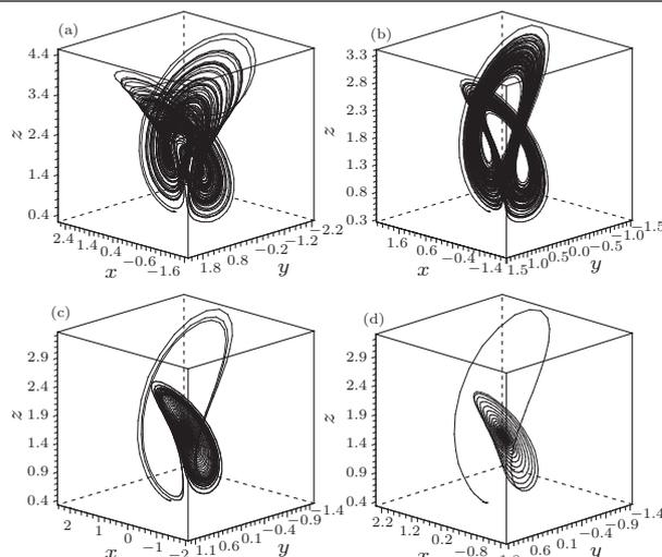
**Fig. 3.** The fractional-order Chen system with conditions:  $\alpha = 1, \alpha = 0.87, \alpha = 0.86, \alpha = 0.85$ .
