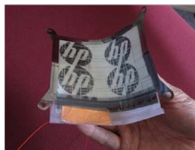
Figure 1: 160X120 pixel e-Ink based display with 500 \mu m pixel pitch being developed for the Army
