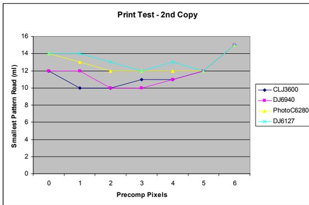
**Figure 3.** 2<sup>nd</sup> Generation copy tests – Smallest symbol (in mils) read for number of pre-compensated pixels.
