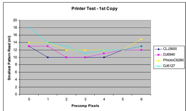
**Figure 2.** 1<sup>st</sup> Generation copy tests – Smallest symbol (in mils) read for number of pre-compensated pixels.
