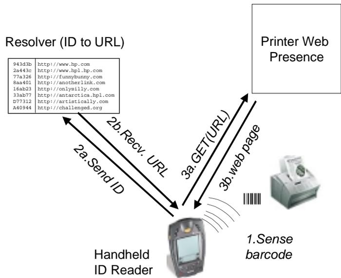
Figure 2. Physical sensing of a printer's web presence.
