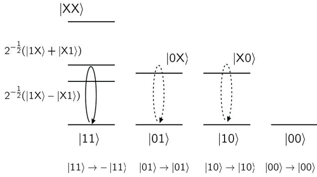
FIG. 1: Schematic of the energy level structure of two resonantly coupled QDs, showing its dependence on the spin state of the excess electron on each dot. When the spins are both in state  $|1\rangle$  an energy shift of the single exciton states occurs due to their Förster coupling. Hence a phase shift may be accumulated using a laser resonant with the dipole allowed transition. This does not occur for any of the other states shown due to the Pauli blocking mechanism.
