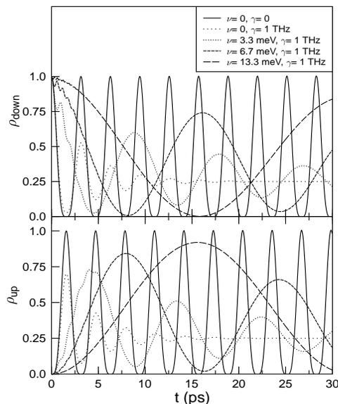
FIG. 3: Population of the state of a single qubit during the proposed  $X$ -rotation gate induced by a two-laser Raman transition. Various values of the exciton decay rate  $\gamma$  and laser detuning  $\nu$  are shown with  $\omega_a = 2$  eV, and  $\Omega = 1.33$  meV for both lasers.
